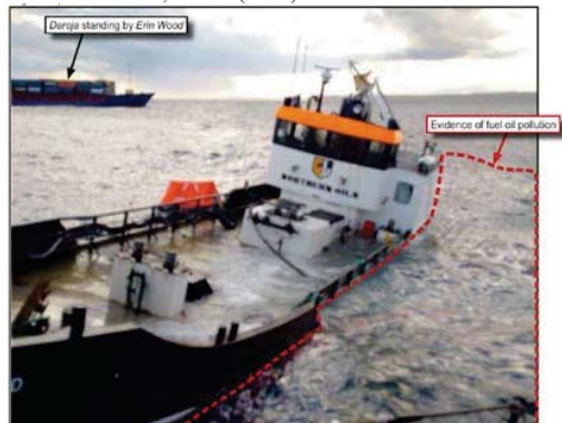
Fig. 2. Erin Wood after the collision as seen from the Peterhead lifeboat, including evidence of fuel cargo pollution, MAIB (2016).
