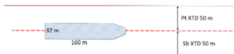
Figure 3: Cross-track distance (XTD), is set to a number of meters on the port and starboard side of the dotted track line. The corridor can then be automatically checked in ECDIS for under-keep clearance. An alarm can also be set to sound if the vessel leaves the corridor.
