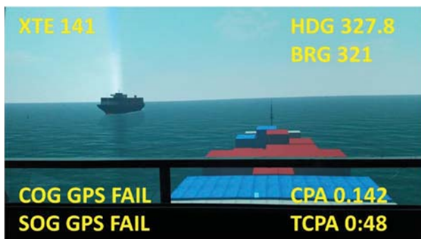
Fig. 5. GlassNav™ display superimposed on a view of the simulated transit.
