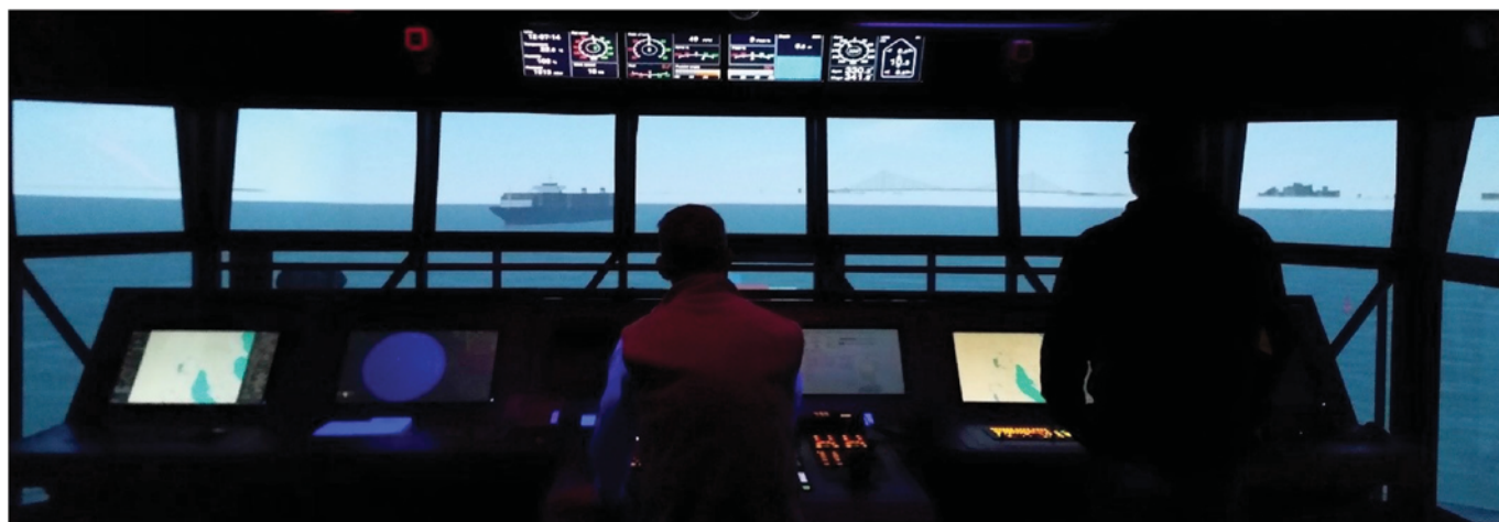
Fig. 2. Simulated bridge showing conventional displays.
