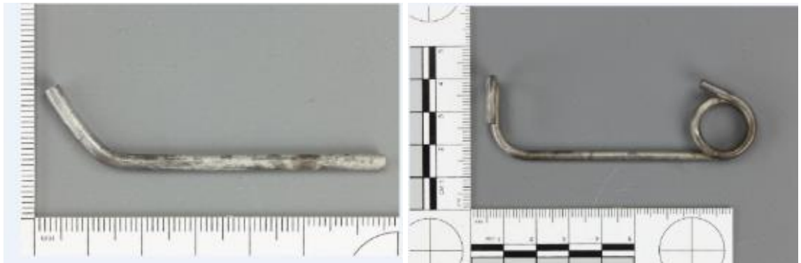
Figure 62: Two segments of safety pins found near the rotor mast. Metallurgical examination proved these to be from two different pins. Photo: AIBN/QinetiQ
