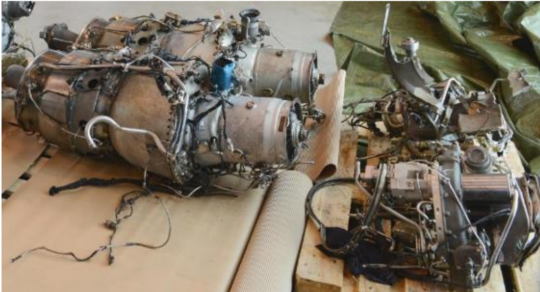
Figure 23: The engines at the AIBN hangar. They had similar damage to a large extent. Both intake sections (Module M01) which had separated from the front part of the engines can be seen to the right of the photo. Photo: AIBN
