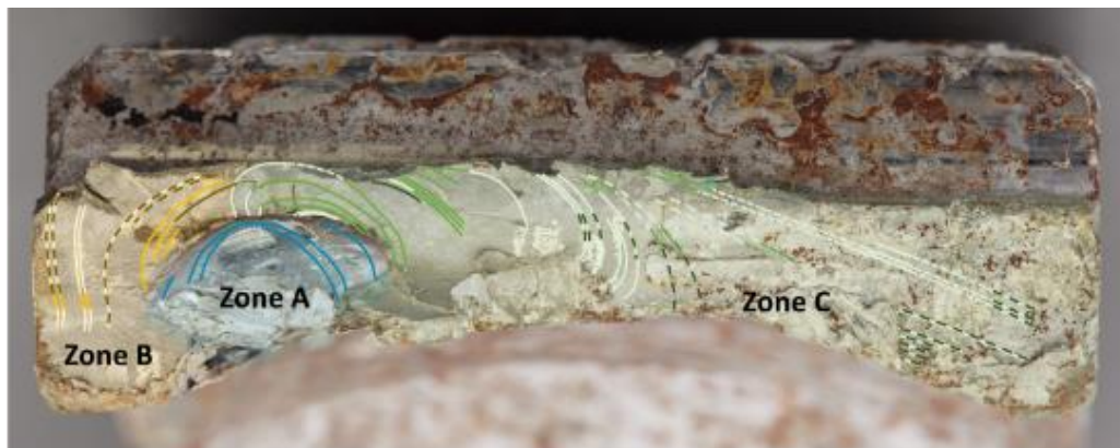
Figure 31: The fracture surface divided into three different zones. The macro marks/features observed are indicated: solid line – well defined, dashed line – less well defined. Photo: AIBN/QinetiQ
