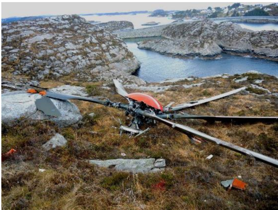
Figure 24: The main rotor and rear suspension bars as found on the island Storskora. Photo: AIBN
