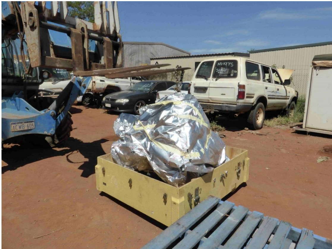
Figure 14: The MGB in the transport container without the damaged top after the ground transport accident 13 March 2015. Photo: Airbus Helicopters
