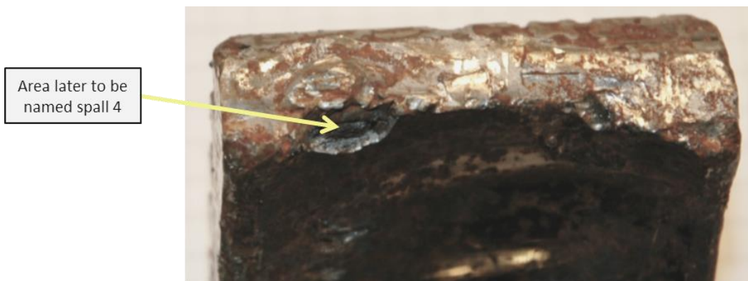
Figure 28: The fracture surface to the left in Figure 27. This surface appeared not to be ductile overload, but possibly fatigue. Photo: AIBN/NDL
