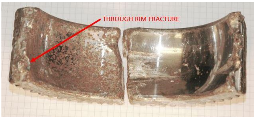
Figure 27: The two segments of the fractured second stage planet gear (serial number M4325). The fatigue fracture through the rim (through-thickness fracture) started in the outer upper race of the planet gear wheel where the red arrow is pointing (spall 4). Photo: AIBN/NDL
