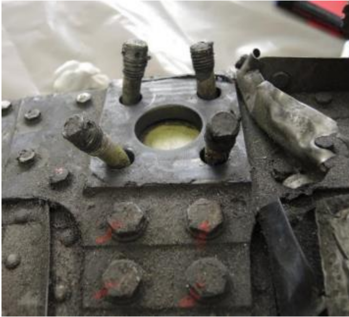
Figure 65: The four bolts from the lower forward fuselage fitting protruding from the support plate. Photo: AIBN
