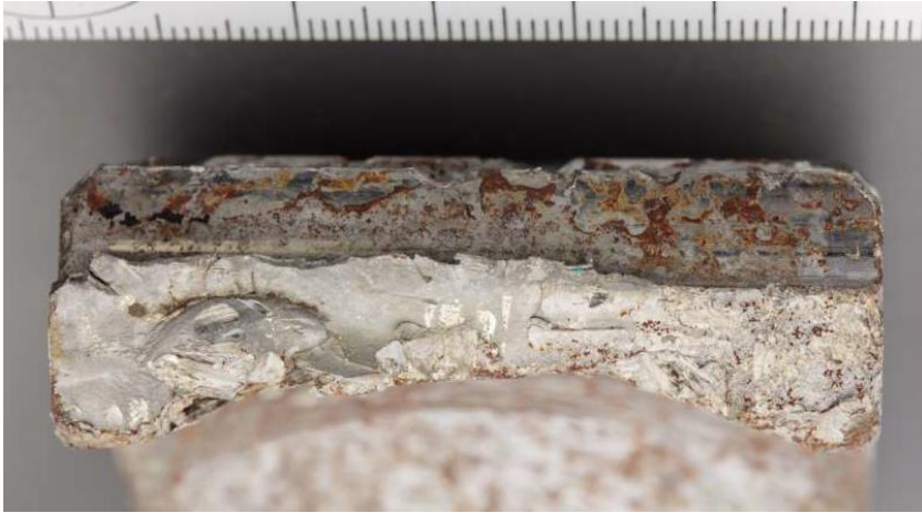
Figure 30: The cleaned through-thickness fracture surface. Macro marks (beach marks) are visible towards the upper edge of the gear (left hand side in photograph). Photo: AIBN/QinetiQ
