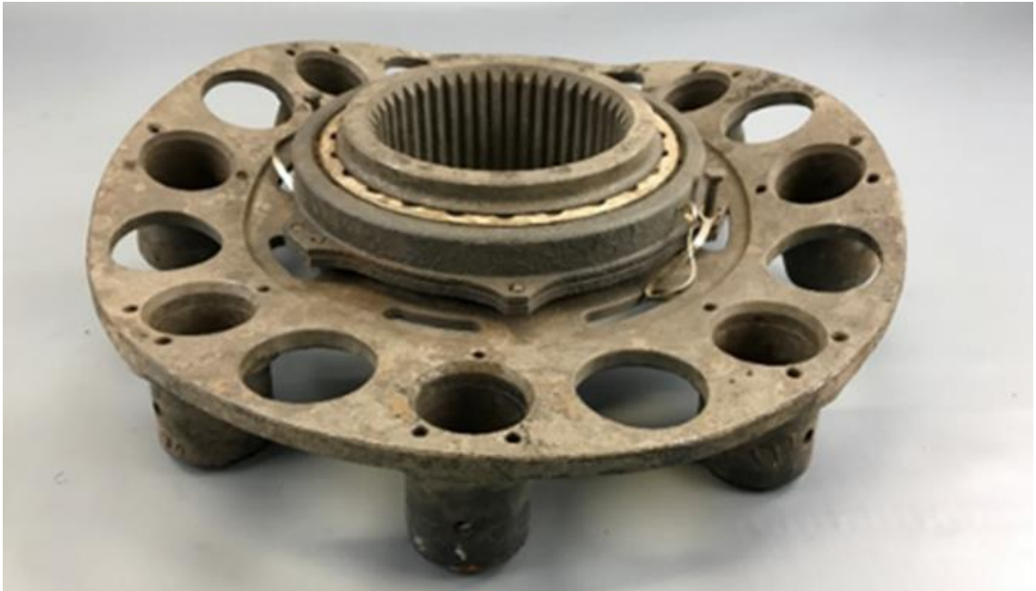
Figure 54: The second stage planet carrier found in February 2017 shown after cleaning. The lower mast bearing is shown on top of the carrier. Photo: AIBN/QinetiQ
