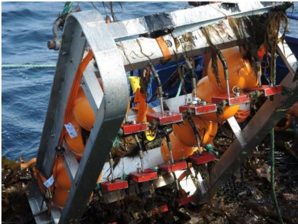
Figure 76: The magnetic sledge being retracted from the sea. Photo: AIBN
