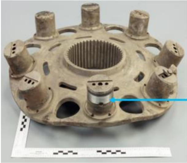
Figure 52: The second stage planet carrier found in February 2017 shown after cleaning. The inner race of the fractured second stage planet gear has been removed from stub shaft number 3 in front. Photo: AIBN/QinetiQ
