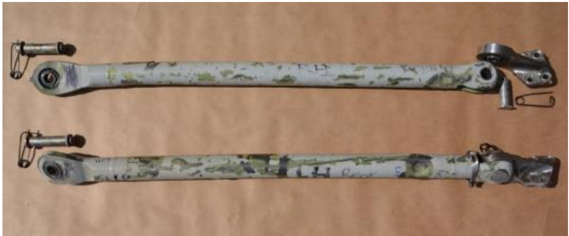
Figure 61: Left and right aft suspension bars with clevis pins, safety pins (only one shown in each position) and fuselage fittings. Both suspension bars have indentations from gear teeth. Photo: AIBN
