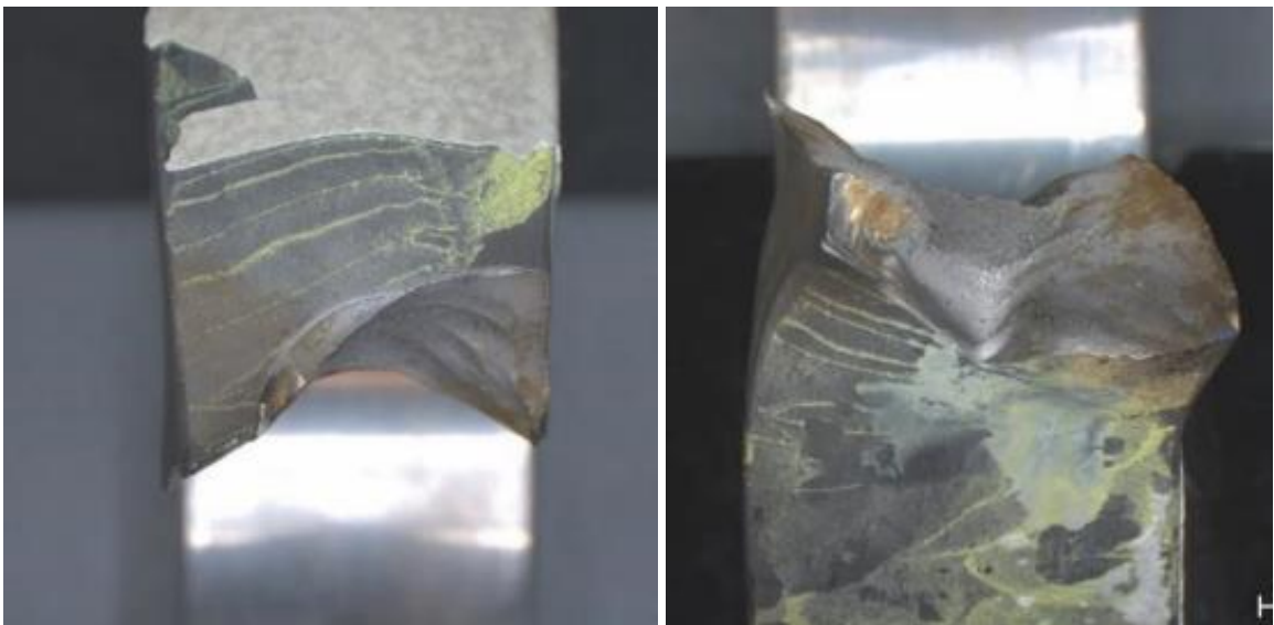
Figure 64: Upper forward suspension bar, mounting lug. Top fracture viewed from above (left photo). Bottom fracture viewed from below (right photo). Photo: AIBN/QinetiQ
