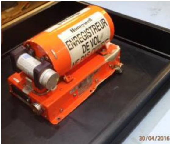
Figure 15: CVFDR from LN-OJF as received at the AAIB. Photo: AIBN
