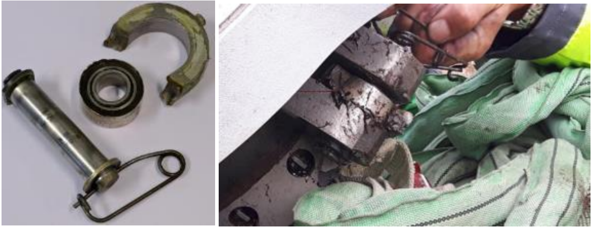
Figure 63: Upper forward suspension bar, part of the mounting lug, the bearing, the clevis pin (with only one of the two safety pins) and the safety pins. Here shown both as found at the rotor mast (right photo) and dismantled (left photo). Photo: AIBN
