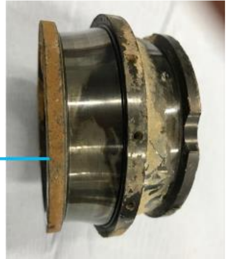
Figure 53: The inner race of the fractured planet gear after cleaning of the upper race (left in photo). Position on the carrier is given by the arrow. Photo: AIBN/QinetiQ
