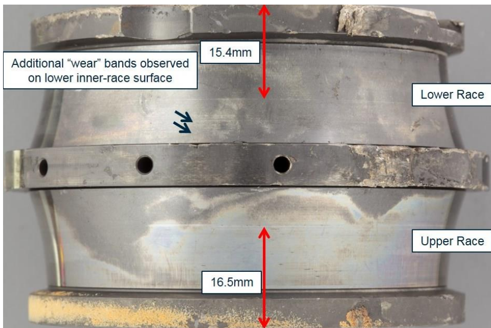
Figure 56: Circumferential ‘wear’ bands on the second stage planet gear inner race observed on both upper and lower race surfaces after cleaning. Photo: AIBN/QinetiQ
