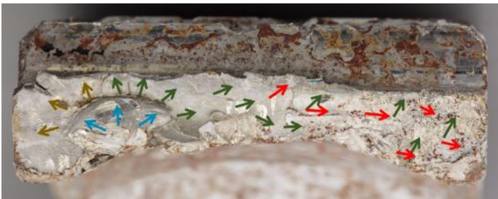
Figure 32: Crack propagation directions concluded from macro mark orientations in zones A (blue), B (brown) and C (green). Propagation in zone C concluded from striation and micro-crack orientations is shown by the red arrows. Photo: AIBN/QinetiQ
