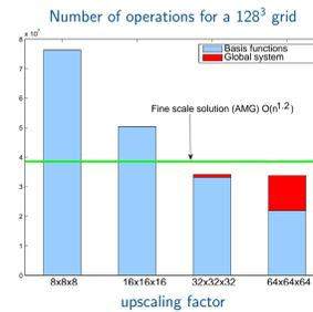
The plot shows that once the basis functions have been computed, the cost of each new pressure solution is relatively low.
