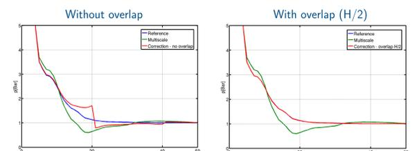
The figures show the multiscale solution in the left half of the reservoir before and after the correction step compared with the fine-grid solution. Using overlap in the domain decomposition method is essential to correct the errors at coarse-grid interfaces.
