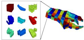
2. Postprocess to ensure all blocks are connected and detect all connections between adjacent gridblocks.
