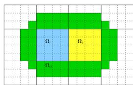
$\Omega_i$  and  $\Omega_j$ : two gridblocks that are connected via a single interface in the coarse grid,  $\Omega_{ij}$  a single-connected domain that contains the two
