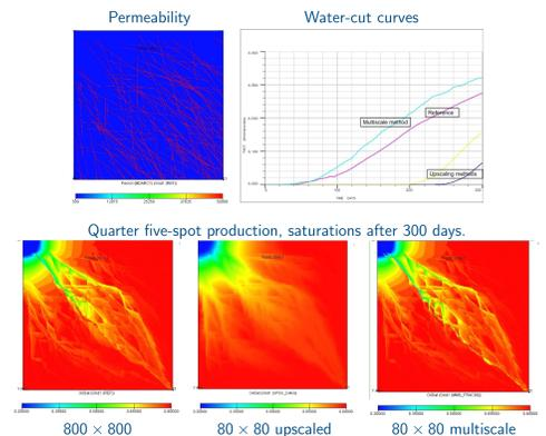
More details: J. R. Natvig et al. Multiscale mimetic solvers for efficient streamline simulation of fractured reservoirs. SPE 119132, 2009 RSS.
