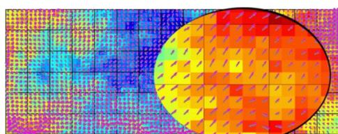
Coarse grid: pressure and fluxes. Fine grid: fluxes
