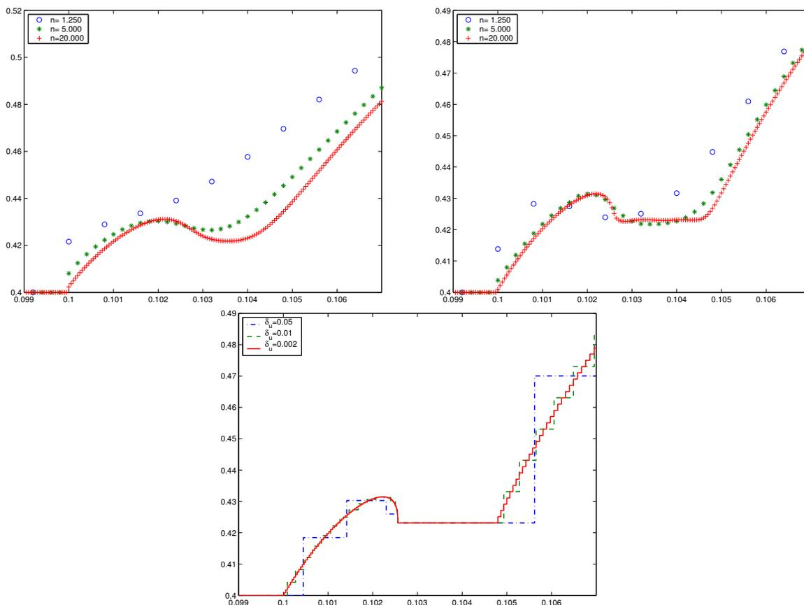
FIGURE 13. (Example 3) Plot of  $1-S_g$  zoomed in around the  $\mathcal{W}_1$  wave. Approximate solutions computed by first-order upwind (top-left) and second-order central-upwind (top-right) on a grid with  $n$  cells, compared with front-tracking (bottom).
