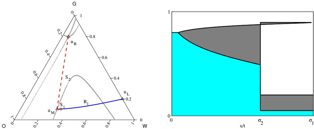
FIGURE 3. Inadmissible Riemann solution with an intermediate state at the detached branch of the Hugoniot locus. Left: Saturation path on the ternary diagram; Right: Saturation profiles showing a nonincreasing sequence of wave speeds ( $\sigma_1 > \sigma_2$ ).
