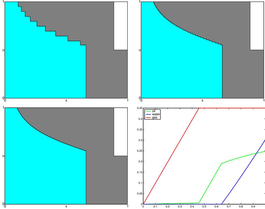
FIGURE 8. (Example 1) Approximate solutions at time  $t = 0.4$  for a water injection in an oil-gas reservoir with  $\delta_u = 0.05, 0.01,$  and  $0.002$ . The bottom-right plot shows cumulative measured production up to time  $t = 1.0$ .
