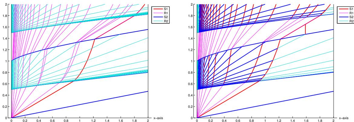
FIGURE 18. (Example 5) Fronts in the  $(x, t)$ -plane for a WAG process computed with  $\delta_u = 0.05$  and no data reduction (left) and with data reduction given by  $\delta_3 = 0.2$  (right).
