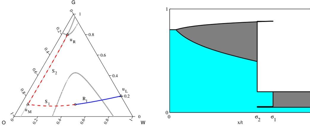
FIGURE 2. Inadmissible Riemann solution using the local branch of the Hugoniot locus. Left: Saturation path on the ternary diagram; Right: Saturation profiles showing a nonincreasing sequence of wave speeds ( $\sigma_1 > \sigma_2$ ).
