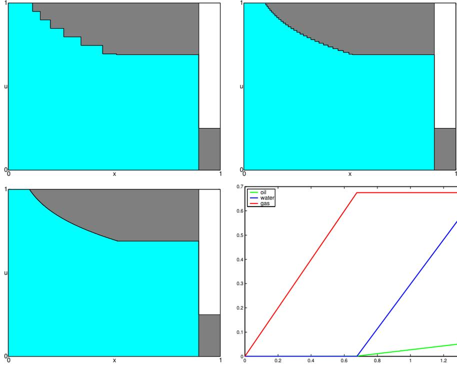
FIGURE 10. (Example 2) Approximate solutions at time  $t = 0.6$  for a solution involving the detached branch of the Hugoniot locus, computed using  $\delta_u = 0.05, 0.01,$  and  $0.002,$  respectively.
