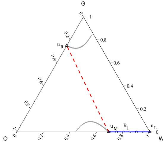
FIGURE 9. (Example 2) Saturation path of the exact solution and the approximate front-tracking solution with  $\delta_u = 0.05$ . The  $\mathcal{S}_2$  shock involves the detached branch of the Hugoniot locus.
