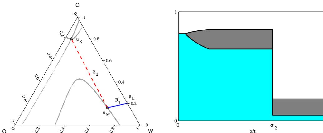
FIGURE 4. Physically correct Riemann solution, where the right state is reached from an intermediate state at the detached branch of the Hugoniot locus. Left: Saturation path on the ternary diagram; Right: Saturation profiles showing a sequence of waves which satisfy the entropy criterion and have increasing speeds.
