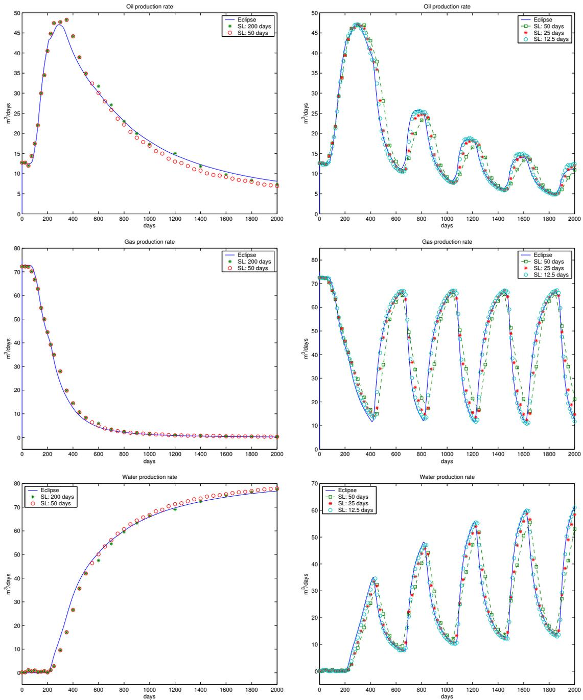
FIGURE 22. Oil, gas, and water rates for water injection (left) and the WAG cycle (right).
