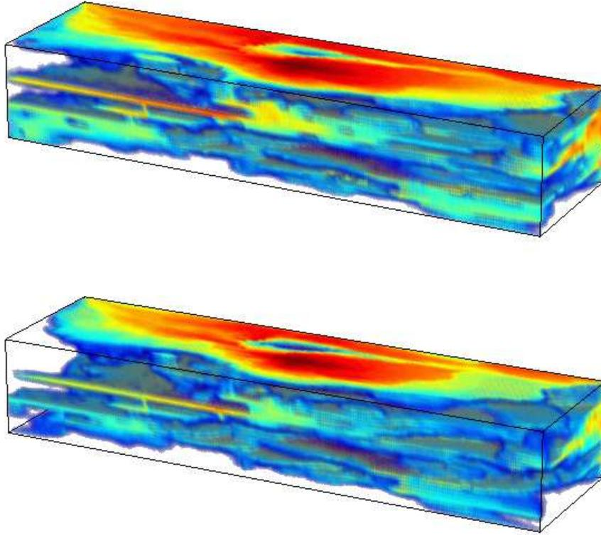
FIGURE 21. Water saturation after 2000 days of production with constant water injection (top) and a WAG cycle (bottom).
