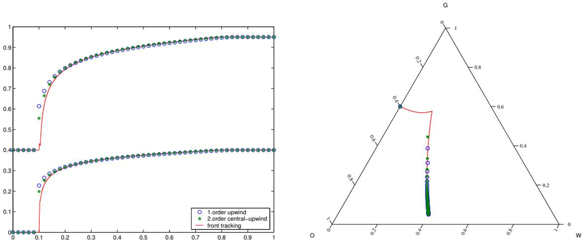
FIGURE 12. (Example 3) Comparison of the front-tracking solution with  $\delta_u = 0.001$  and two finite-volume methods on a grid with  $\Delta x = 1/50$ ; the left plot shows solutions in the  $(x, u)$ -plane and the right plot shows solutions in the ternary diagram.
