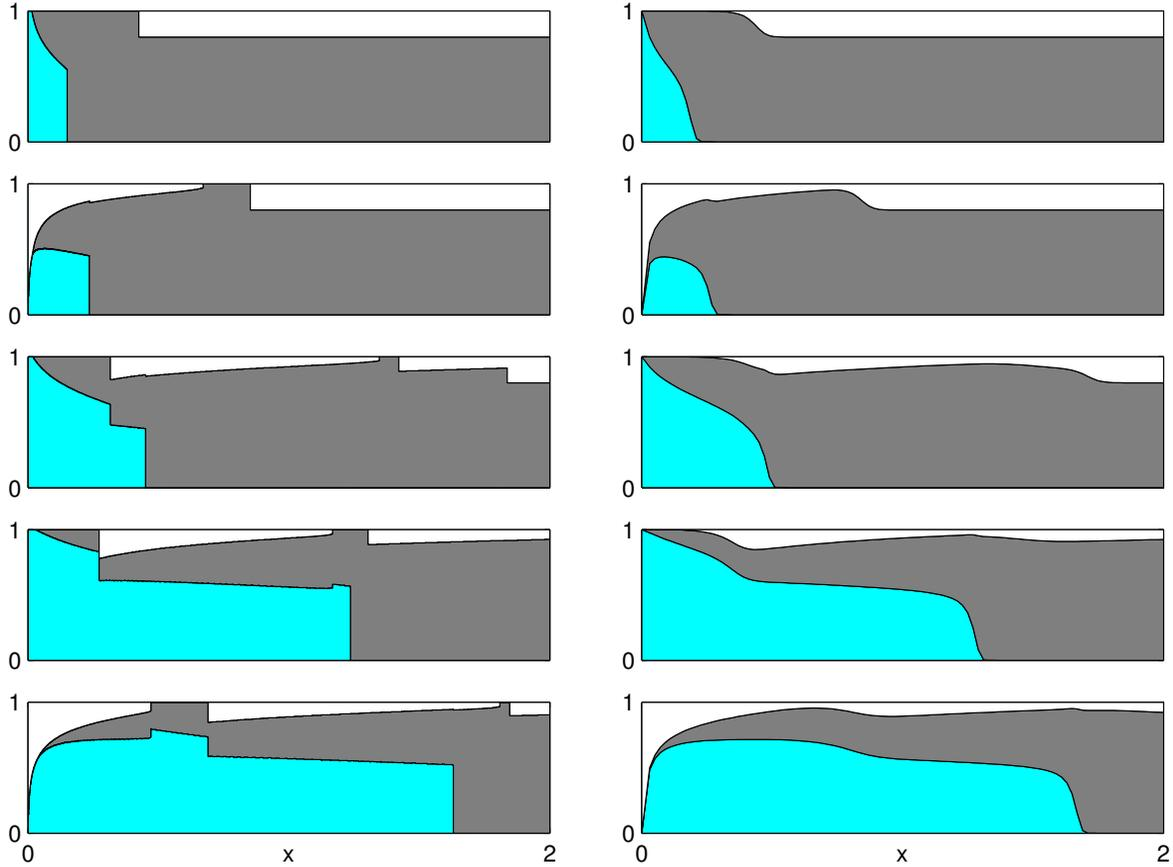
FIGURE 15. (Example 4) Saturation profiles for the one-dimensional WAG process at  $t = 0.1$  (top), 0.2, 0.5, 1.5 and  $t = 2$  (bottom), calculated by: the front-tracking using  $\delta_u = 0.005$  (left), and the first-order upwind method with 100 grid cells (right).
