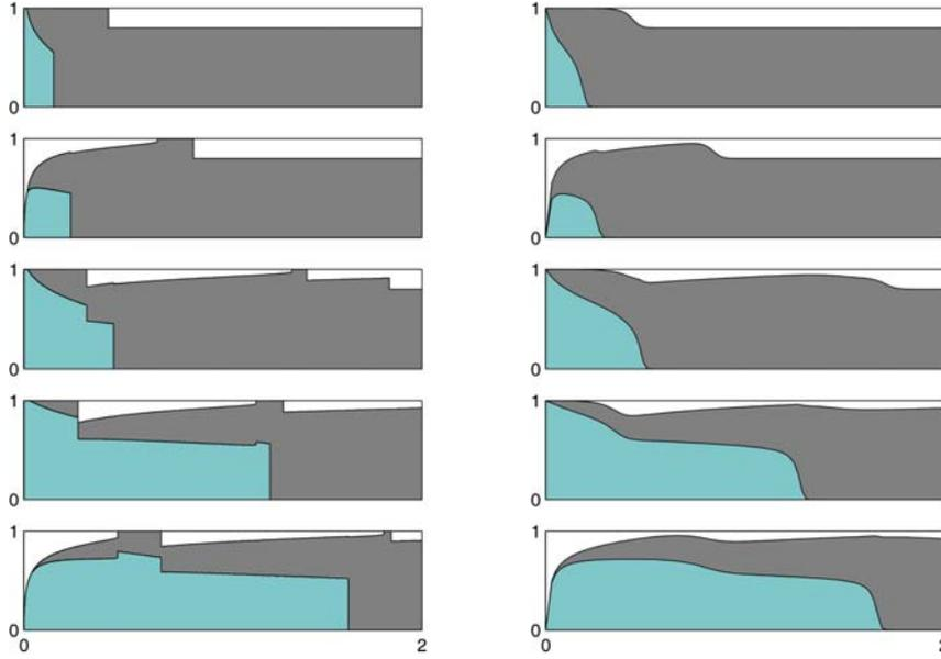
Fig. 3. Saturation profiles at  $t = 0, 0.1, 0.2, 0.5, 1.5$  and  $t = 2$ , calculated by: front-tracking using  $\delta_u = 0.005$  (left), and upwind finite differences with 100 grid cells (right).
