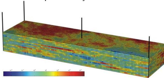
Fig. 5. Logarithm of horizontal permeability and well configuration for the Tarbert formation.
