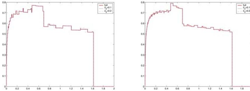
Fig. 4. Water saturation profiles with varying degree of data reduction:  $\delta_u = 0.05$  (left), and 0.025 (right).
