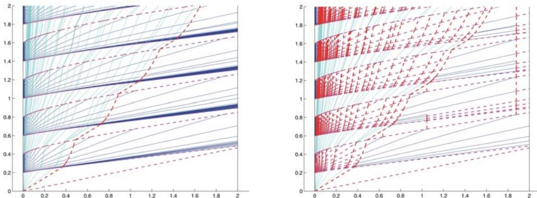
Fig. 2. Fronts in the  $(x, t)$ -plane for the one-dimensional WAG process, using  $\delta_u = 0.05$ . Shocks are shown as dashed lines, whereas rarefactions are solid lines. (Left) Full resolution of all waves with  $\delta_1 = \delta_2 = \delta_3 = 10^{-5}$ . (Right) Data reduction with  $\delta_3 = 0.2$  and  $\delta_1 = \delta_2 = 10^{-5}$ .
