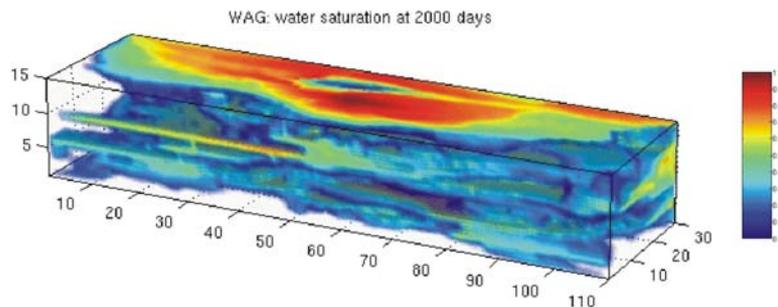
Fig. 6. Water saturation after 2000 days of production with a WAG injection scheme.
