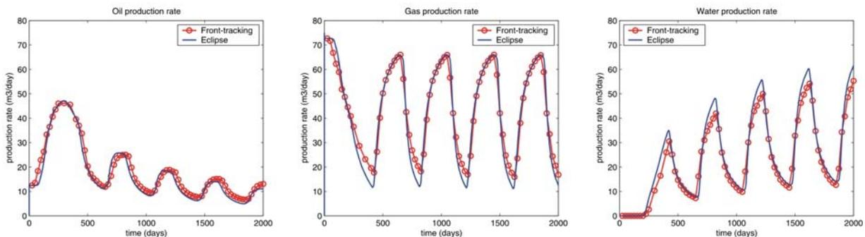
Fig. 7. Oil, gas, and water production rates computed by the front-tracking simulator and Eclipse.
