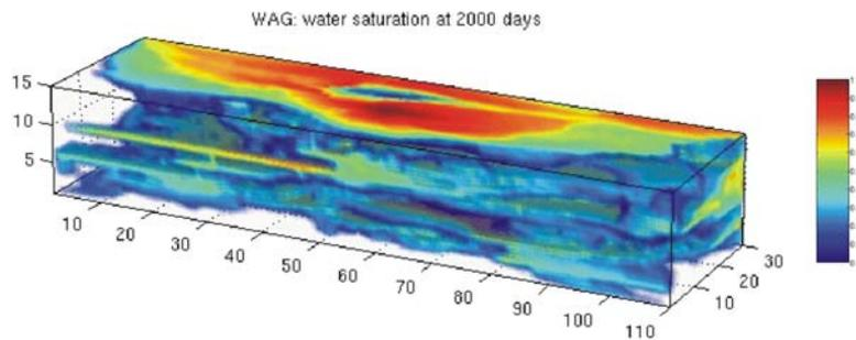
Fig. 6. Water saturation after 2000 days of production with a WAG injection scheme.
