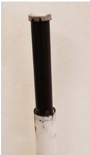
Backbone-segment coated with BGLC-suspension
