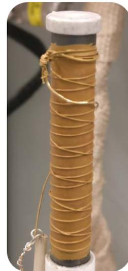
Figure 11 LSM-BCZY27-BCZY27Ni60 cell sealed into alumina riser with Gold as current collector
