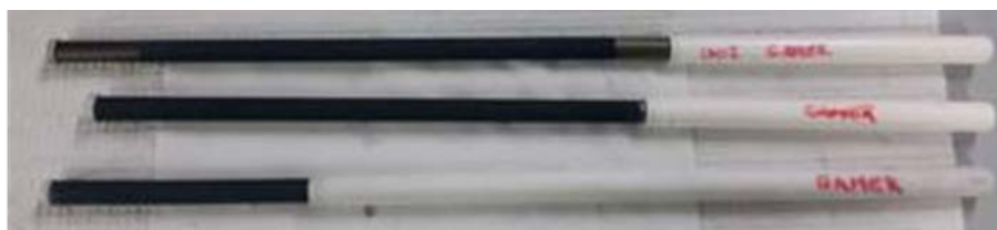
Figure 3. 15 cm and 25 cm long cells cap-sealed and mounted on alumina risers in GAMER for further electrochemical testing
