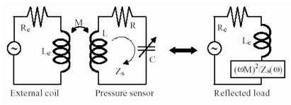
Fig. 3: Equivalent circuit model of the telemetric readout approach.
