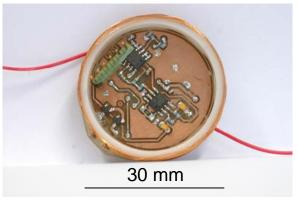
Prototype with a coil antenna
