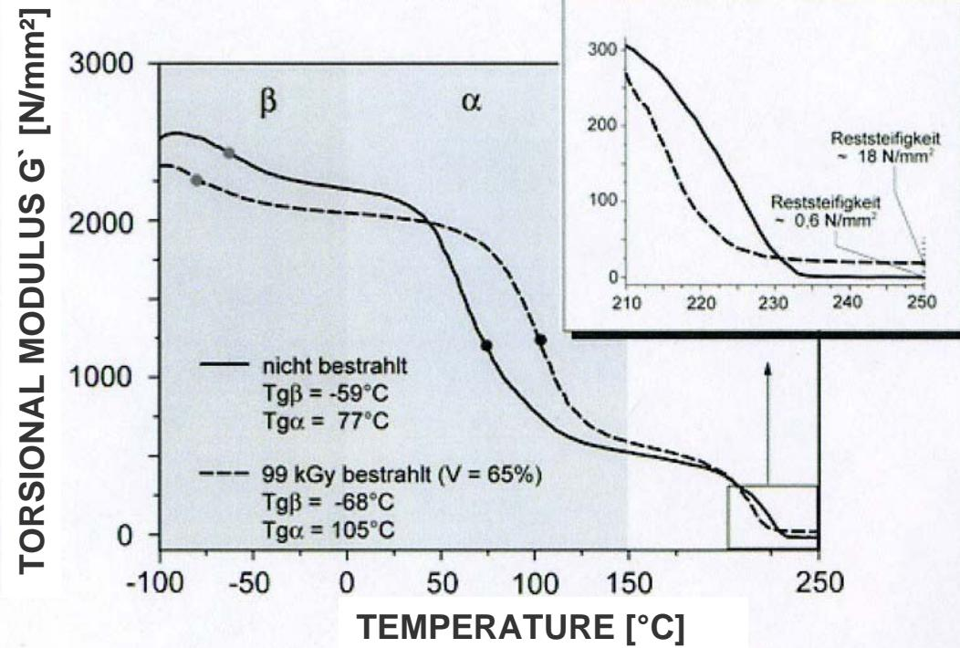
Increasing of glass transition temperature and remaining stiffness by means of crosslinking.
