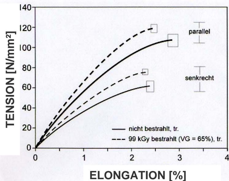
Crosslinking leads to higher tensile strength and reduced elasticity.
