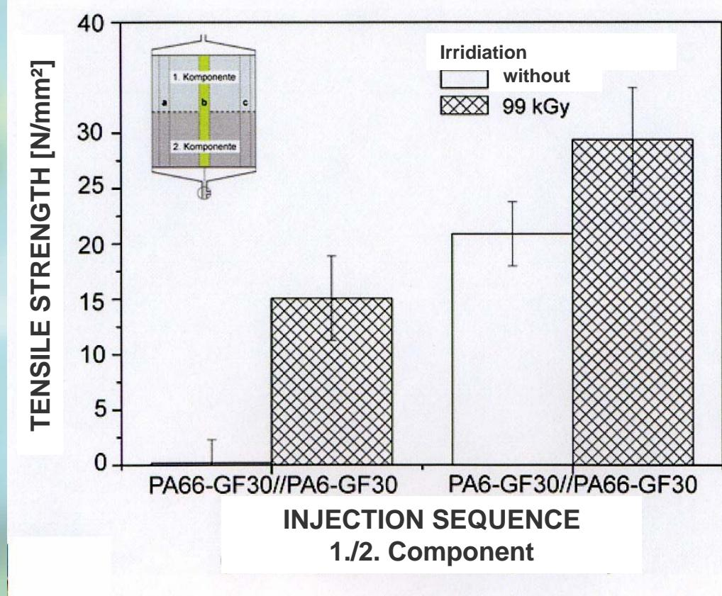
Tensile Test in accordance to DIN 2156; 2mm/Min;  $\sigma_{\max}$
