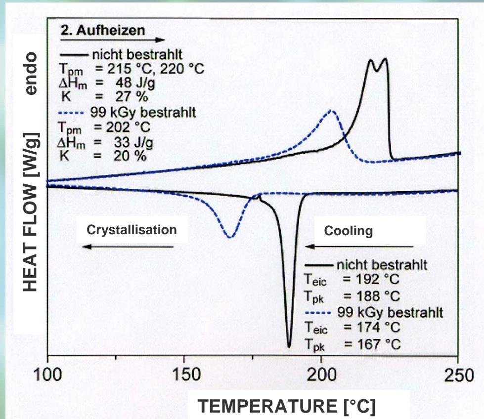
The crystallinity is disturbed by the crosslinked areas. The result is a lower crystallisation temperature and reduction of heat content!
