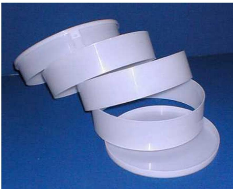
*Fig. 1. A photograph of the container after cutting it into five segments, in order to quantify the material distribution.*
