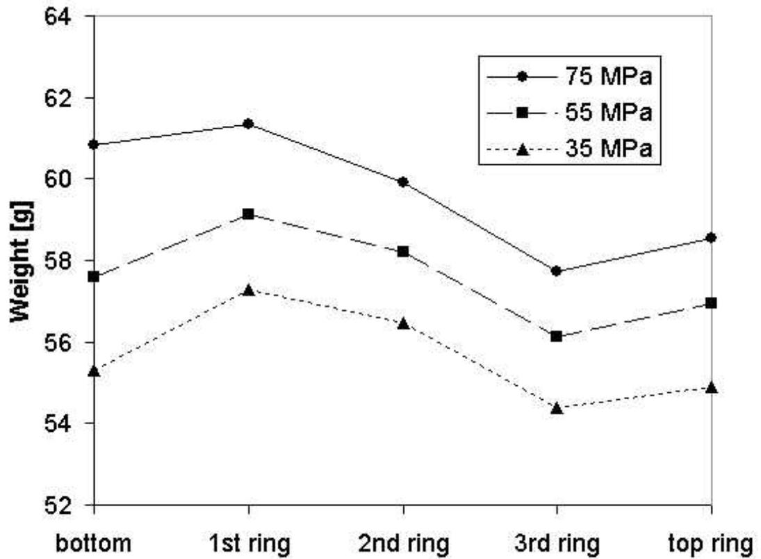
Fig. 2. Material distributions for different packing pressures. Data for BE375P with packing time 1.5 s.
