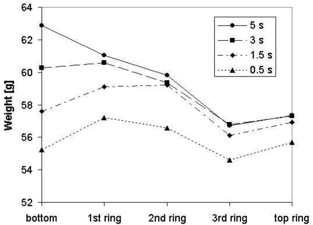
Fig. 3. Material distributions for different packing times. Data for BE375P with packing pressure 55 MPa.
