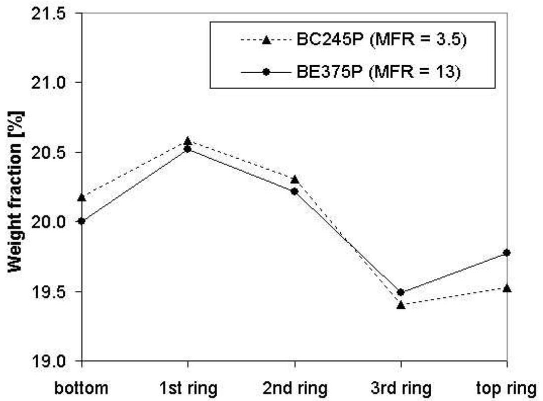
*Fig. 5. Material distributions for different MFR values. The packing pressure and time were 55 MPa and 1.5 s, respectively.*
