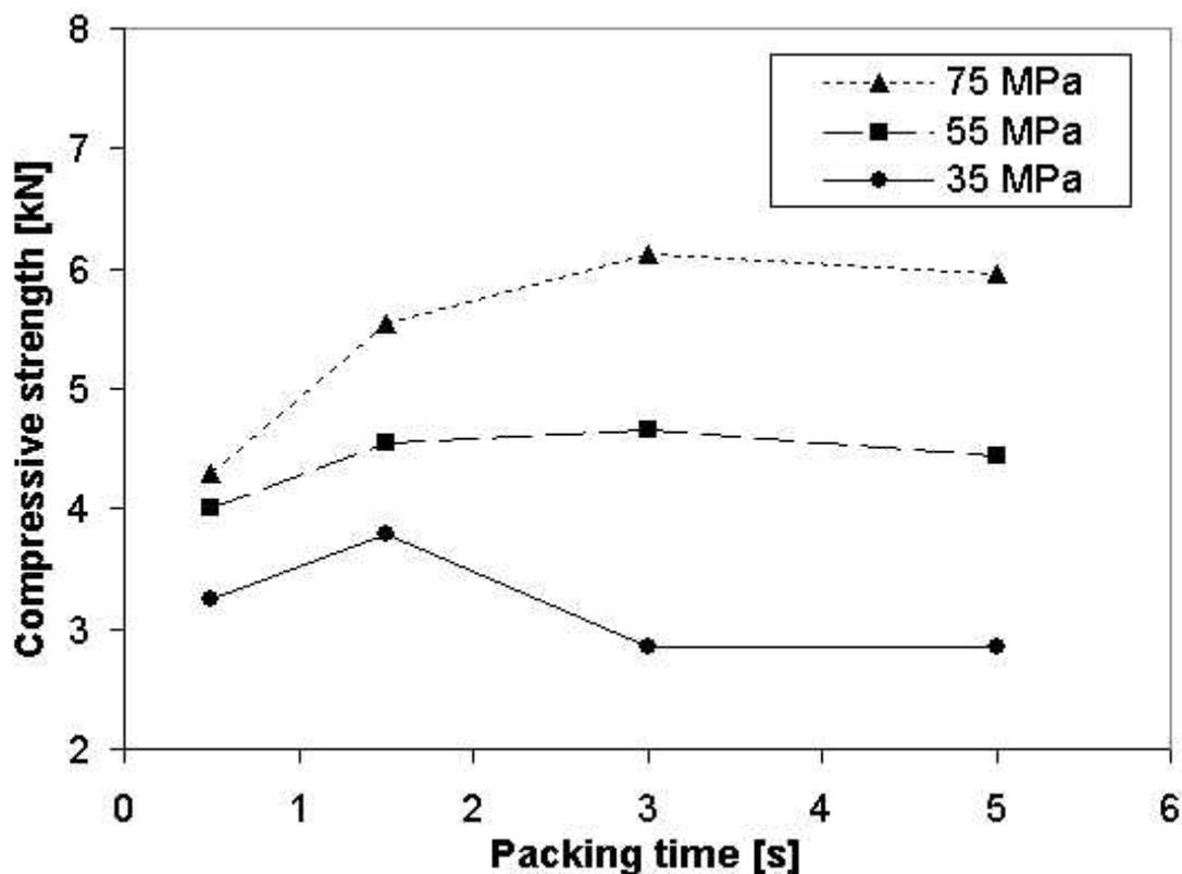
Fig. 8. Compressive strength of BE375P for different packing times and pressures.
