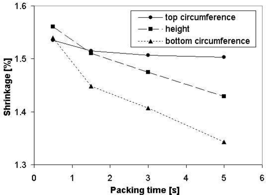
Fig. 7. Shrinkage of BE375P vs. packing time, with 55 MPa packing pressure.
