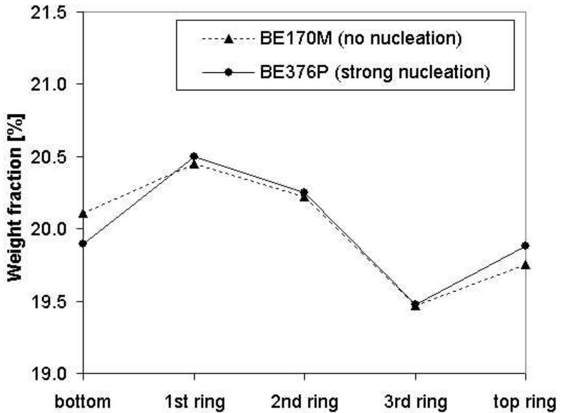
*Fig. 6. Material distributions for different degrees of nucleation. The packing pressure and time were 55 MPa and 1.5 s, respectively.*
