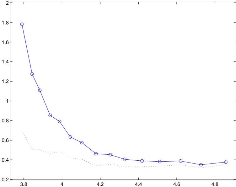
FIGURE 30.21. Sphere: approximative drag coefficient as a function of the 10-logarithm of the number of mesh points in space.
