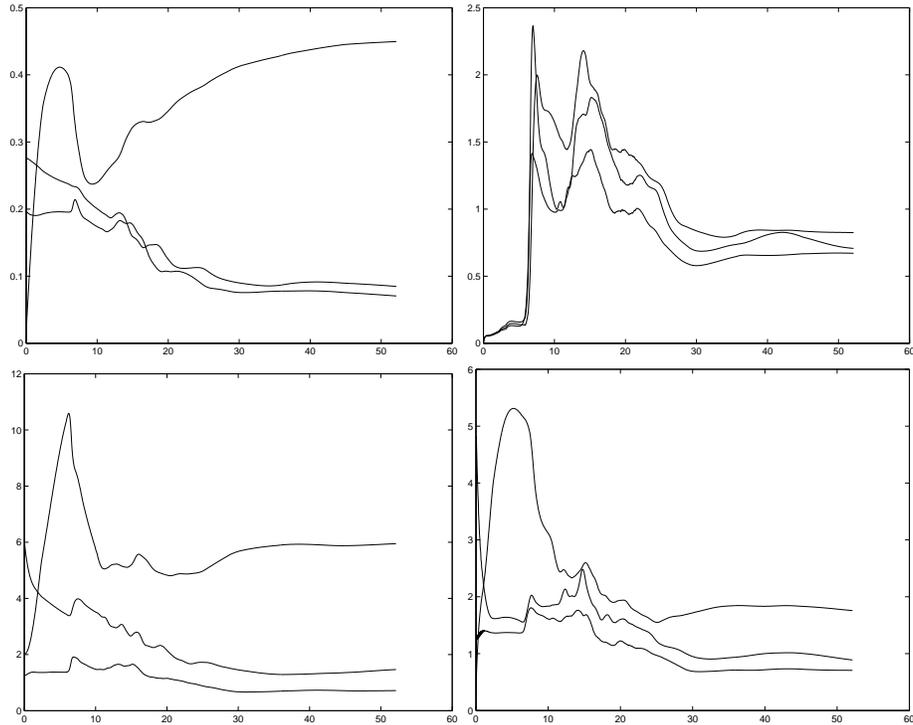
FIGURE 34.12.  $x_3$ -periodic Couette flow ( $\kappa\nu = 0.5$ , random force perturbation): Perturbations  $\|\varphi_i\|$  as functions of time (upper left), derivatives  $\|\partial u_i/\partial x_1\|$  (upper right),  $\|\partial u_i/\partial x_2\|$  (lower left), and  $\|\partial u_i/\partial x_3\|$  (lower right) as functions of time.
