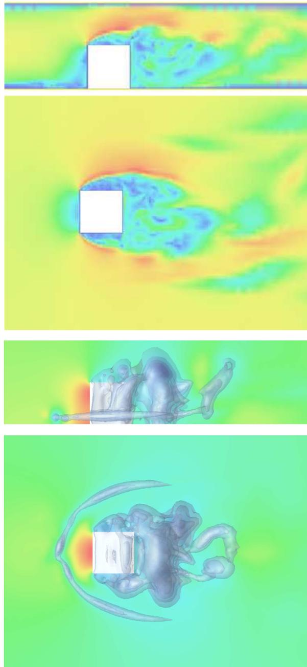
FIGURE 30.1. Surface mounted cube: Magnitude of velocity (upper), and pressure color map, with isosurfaces for negative pressure, illustrating the horse shoe vortex.
