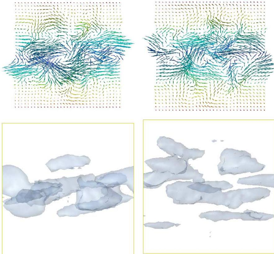
FIGURE 34.23. Slowest decaying modes from a uniformly distributed random perturbation, in the  $x_2x_3$ -plane at  $x_1 = 0.25$  (upper left) and  $x_1 = 0.75$  (upper right), isosurfaces for  $|u| = 0.015$  in the  $x_1x_2$ -plane (lower left) and in the  $x_1x_3$ -plane (lower right).
