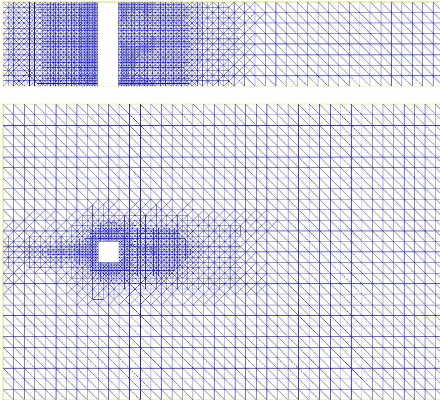
FIGURE 20.2. Computational mesh in the  $x_1x_2$ -plane (upper) and the  $x_1x_3$ -plane (lower).
