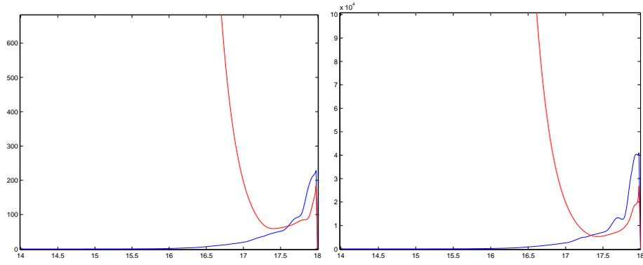
FIGURE 20.10. The  $L_2$ -norm of the dual velocity (left) and dual velocity gradient (right), linearized at  $U(0) = \nabla\phi$  and turbulent flow respectively.
