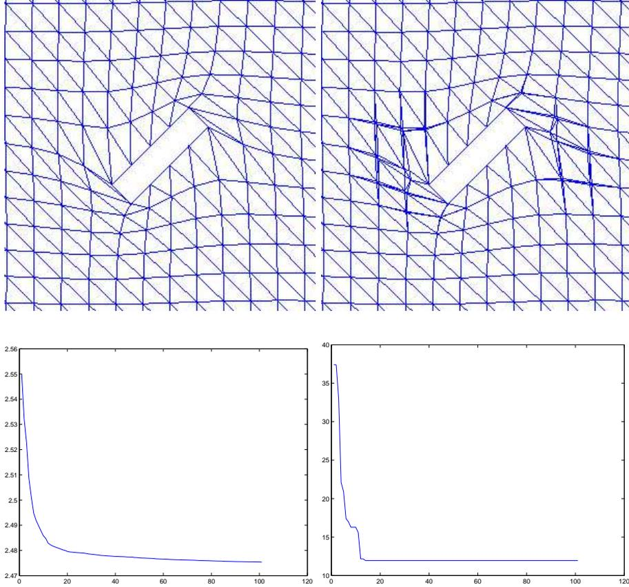
FIGURE 29.2. Rotated object mesh before (upper left) with Laplacian mesh smoothing, and after 100 iterations of the local optimization algorithm (upper right). The weighted  $l_2$ -norm (lower left), and the max-norm (lower right) of the square root of the condition numbers of  $A^T A$  as functions of number of iterations.
