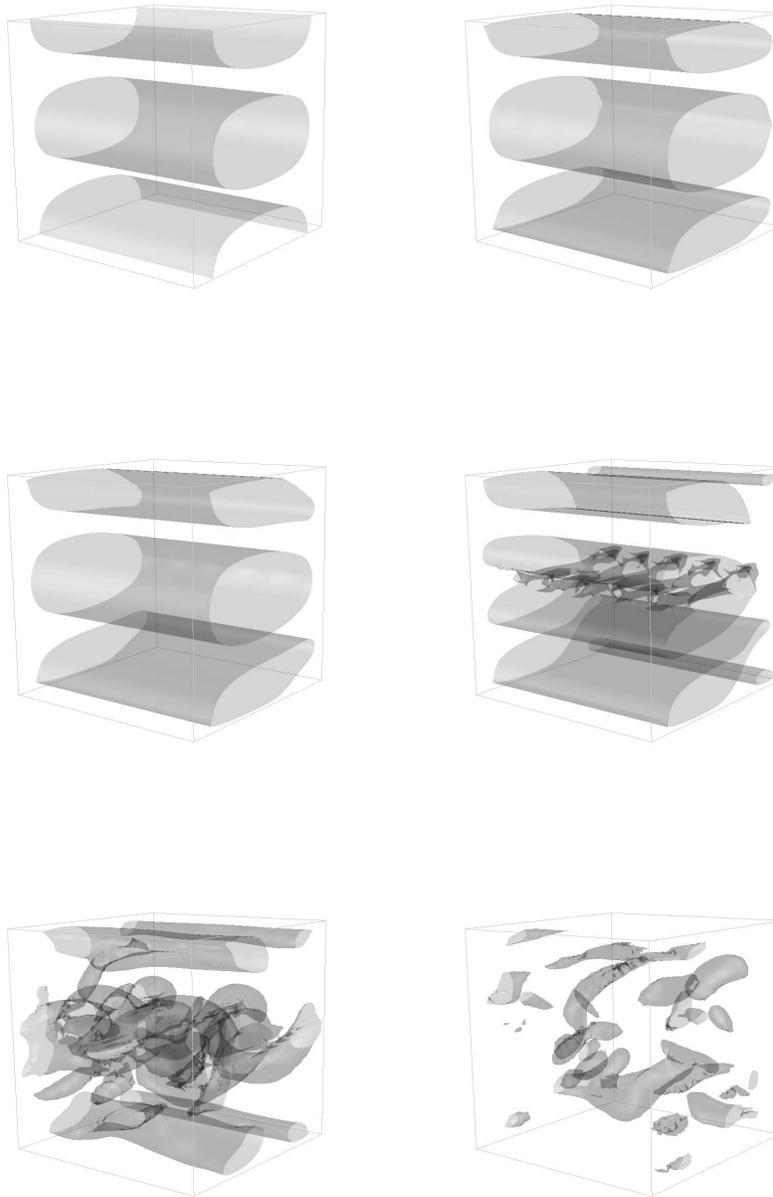
FIGURE 34.9. Transversal velocity isosurfaces for  $|u_3| = 0.2$  in Couette flow ( $\kappa\nu = 0.5$ ) for  $t = 0, 5, 10, 15, 20, 30$
