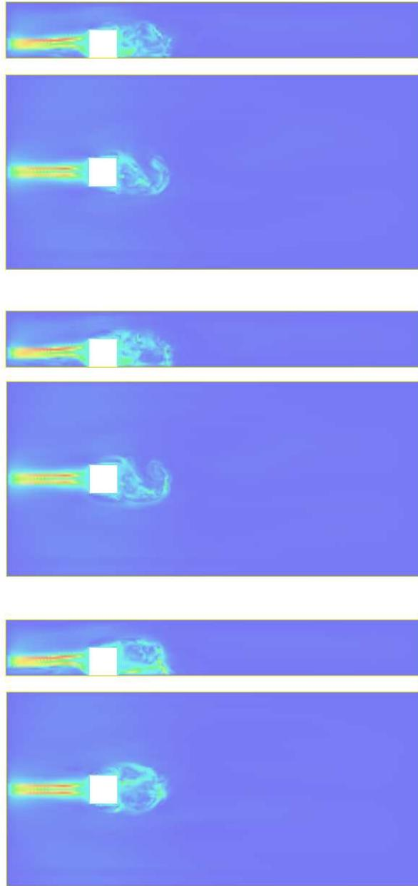
FIGURE 14.6. Surface mounted cube: snapshots of the dual velocity  $|\varphi_h|$  sampled 4 times per time unit (upper), 2 times per time unit (middle), and once per time unit (lower), corresponding to “4”, “2”, and “1”, in Table 14.1, in the  $x_1x_2$ -plane at  $x_3 = 3.5H$  and in the  $x_1x_3$ -plane at  $x_2 = 0.5H$ .
