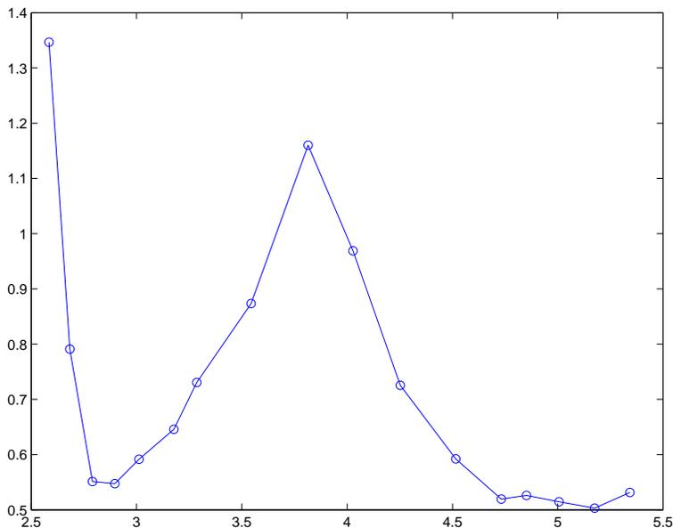
FIGURE 20.15. The mean value of the dissipation intensity of G2 in the turbulent wake of the flow around a surface mounted cube (see Chapter 30), vs  $\log_{10}$  of the number of mesh points.
