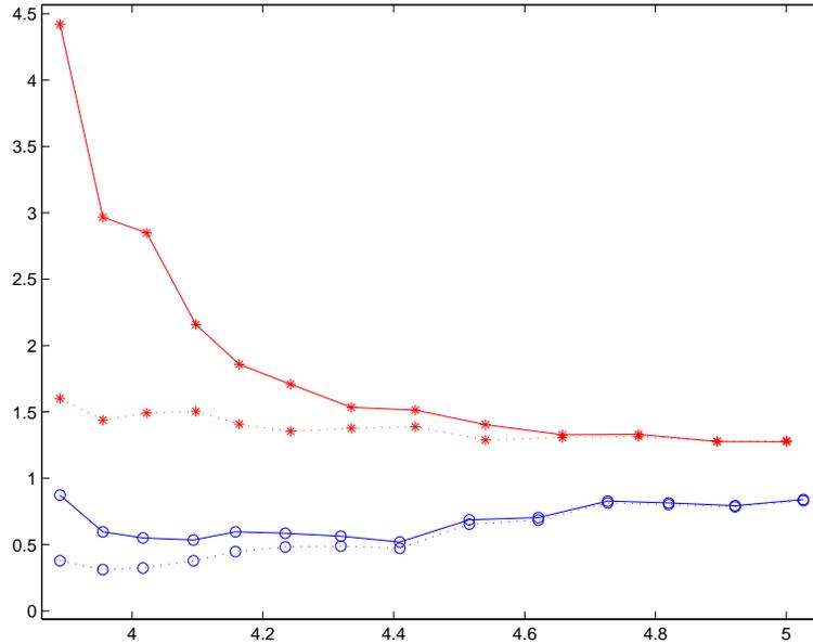
FIGURE 32.6.  $\bar{c}_D^h$  vs  $\log_{10} \# \text{ nodes}$  for the rotating ('\*') and the stationary ('o') cylinder.
