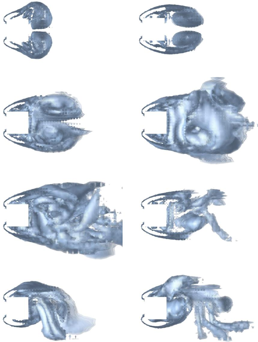
FIGURE 20.9. Magnitude of the vorticity corresponding to zero initial data, for time steps 48,64,96,128,160,704,960,1024.
