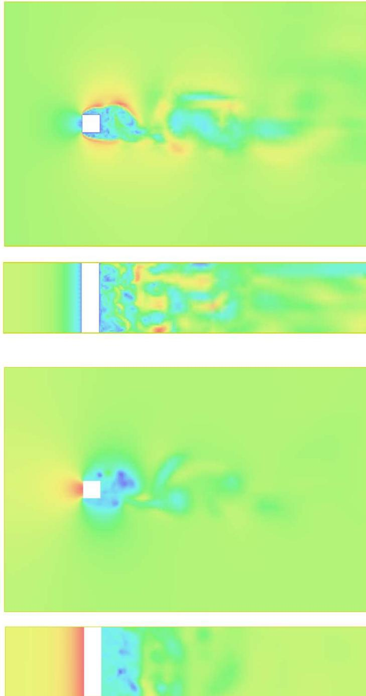
FIGURE 30.5. Velocity  $|U|$  (upper), and pressure  $P$  (lower), in the  $x_1x_2$ -plane at  $x_3 = 2D$ .
