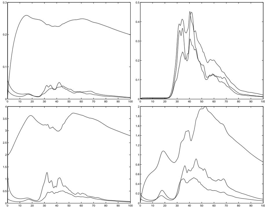
FIGURE 34.10. Couette flow ( $\kappa\nu = 0.1$ ): Perturbations  $\|\varphi_i\|$  as functions of time (upper left), derivatives  $\|\partial u_i/\partial x_1\|$  (upper right),  $\|\partial u_i/\partial x_2\|$  (lower left), and  $\|\partial u_i/\partial x_3\|$  (lower right) as functions of time.
