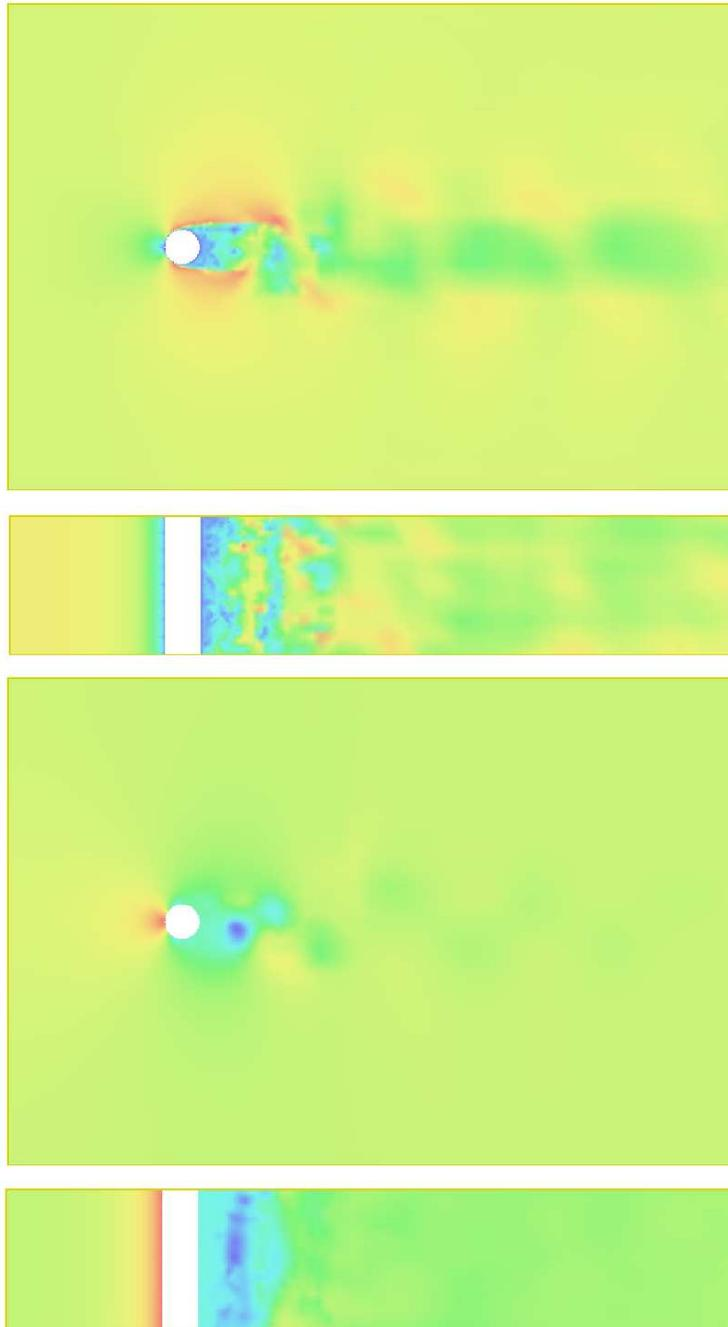
FIGURE 30.13. Circular cylinder at  $Re = 3900$ : magnitude of velocity  $|U|$  (upper), and pressure  $P$  (lower).
