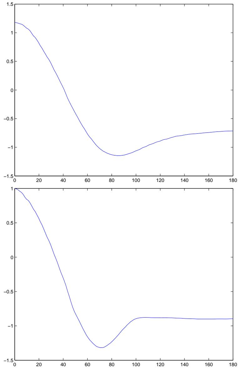
FIGURE 30.16. Circular cylinder: Pressure coefficient  $c_p$  as a function of an angle starting at the stagnation point, for  $Re = 100$  (upper) and  $Re = 3900$  (lower).
