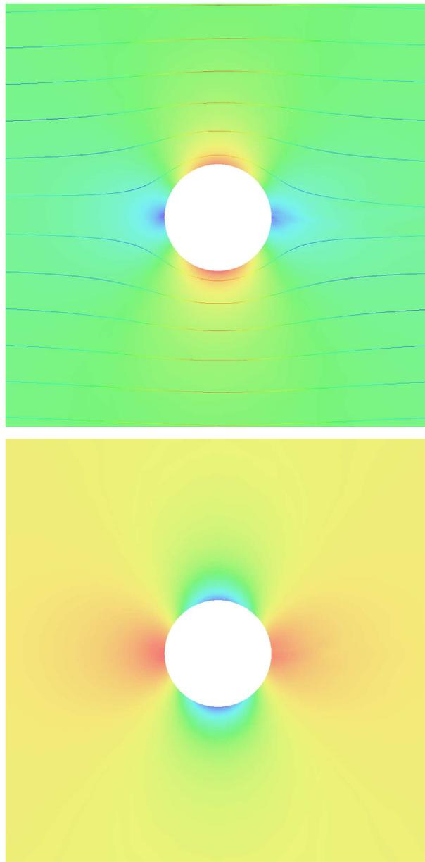
FIGURE 11.1. Flow past a circular cylinder; velocity (upper) and pressure (lower).
