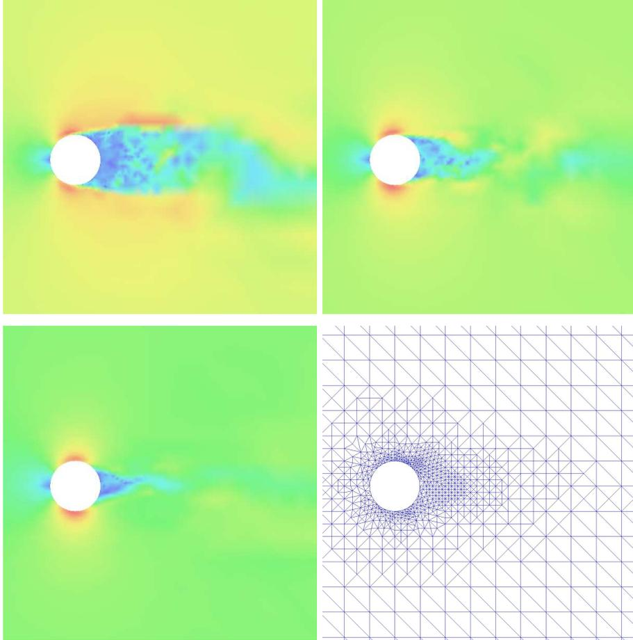
FIGURE 32.4. Drag crisis: magnitude of the velocity for G2 solutions for  $\nu = 0$ ;  $\beta = 2 \times 10^{-2}$  with  $c_D \approx 0.7$  (upper left),  $\beta = 1 \times 10^{-2}$  with  $c_D \approx 0.5$  (upper right),  $\beta = 5 \times 10^{-3}$  with  $c_D \approx 0.45$  (lower left), and the mesh with 80 000 mesh points (lower right), in the  $x_1x_2$ -plane for  $x_3 = 0.2$ .
