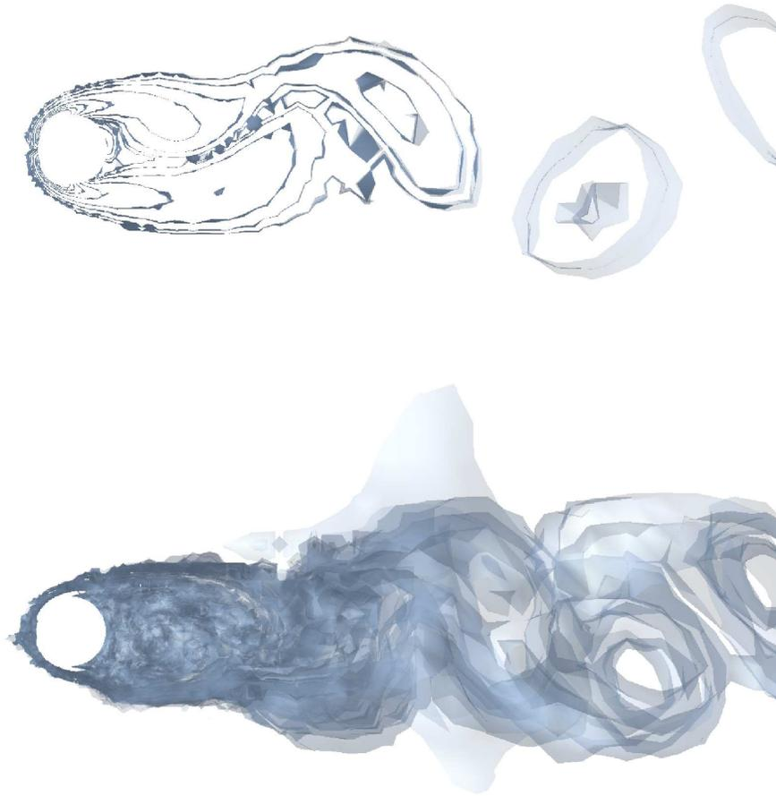
FIGURE 30.14. Magnitude of vorticity isosurfaces for 3,5,10,20,...,100, for a circular cylinder at  $Re = 100$  (upper), and  $Re = 3900$  (lower).
