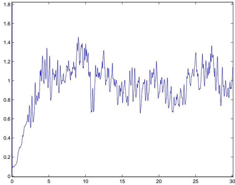
FIGURE 11.6. Time series of  $c_D$  for a G2 solution to the Euler equations.
