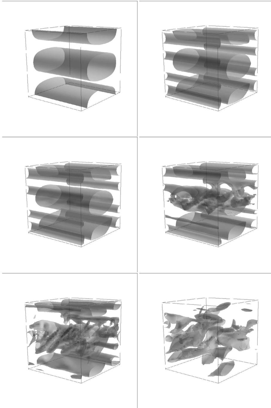
FIGURE 34.15. Transversal velocity isosurfaces for  $|u_3| = 0.2$  in  $x_3$ -periodic Couette flow ( $\kappa\nu = 0.5$ , random force perturbation) for  $t = 0, 5, 6, 7, 10, 20$
