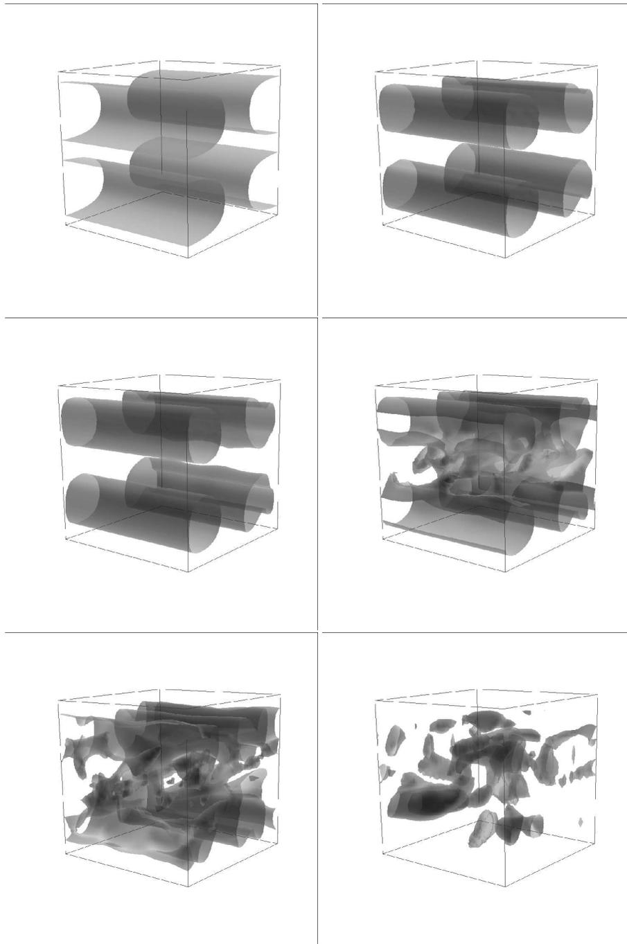
FIGURE 34.14. Transversal velocity isosurfaces for  $|u_2| = 0.2$  in  $x_3$ -periodic Couette flow ( $\kappa\nu = 0.5$ , random force perturbation) for  $t = 0, 5, 6, 7, 10, 20$
