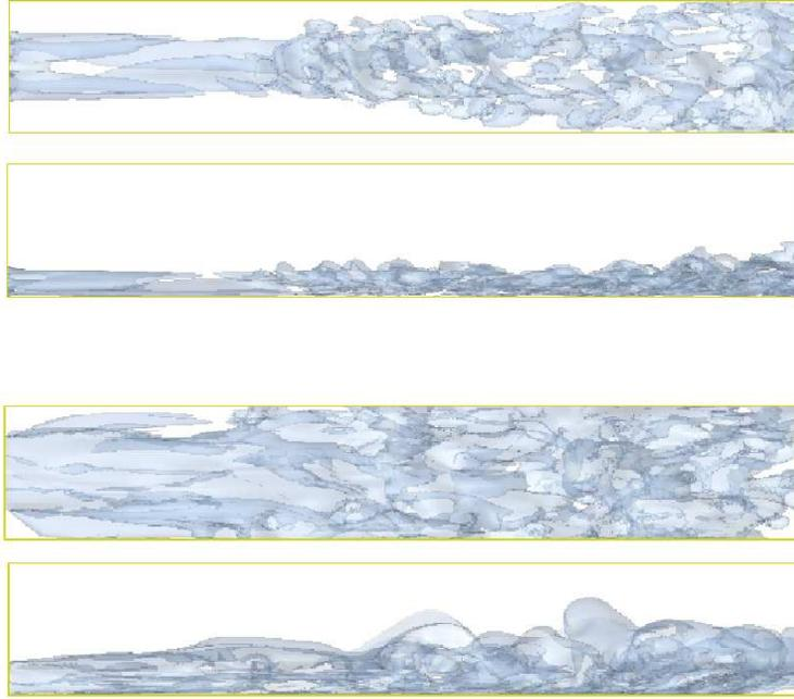
FIGURE 34.24. Isosurfaces for  $|(u_2, u_3)| = 0.06$  for transition to turbulence in a boundary layer computation from Chapter 31, for  $\nu = 10^6$ ,  $l = 6$ , and  $b = 1$ , introducing Taylor-Görtler type perturbations at the inflow of amplitude 0.1 (upper) and 0.5 (lower), resulting in transition further downstream for the lower perturbation.
