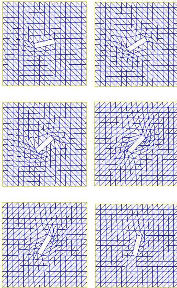
FIGURE 29.4. Box rotation with Laplacian smoothing, for an  $0.25 \times 0.0625 \times 0.25$  object inside a  $1 \times 1 \times 1$  box.
