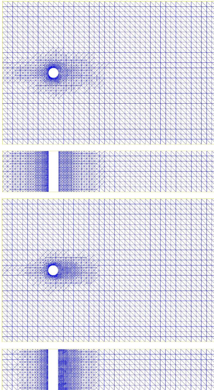
FIGURE 30.19. Circular cylinder: Computational mesh for  $Re = 100$  (upper), and  $Re = 3900$  (lower).
