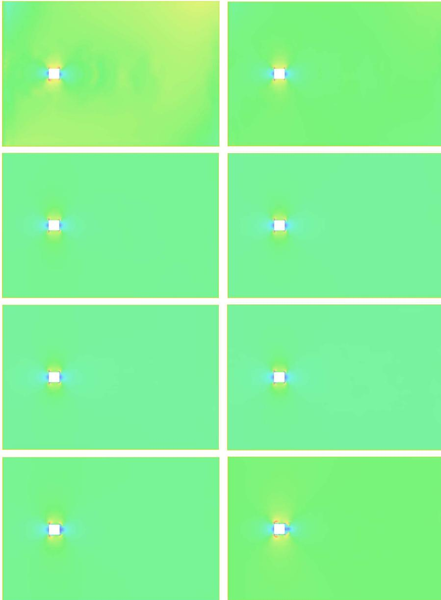
FIGURE 20.3. Magnitude of the computed velocity from initial data  $U(0) = \nabla\phi$ , for time steps no 1,2,4,5,6,7,20,37.
