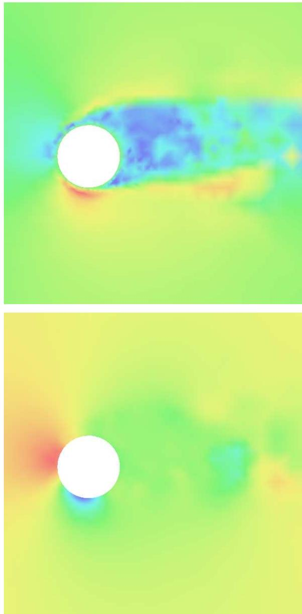
FIGURE 32.5. Asymmetric separation of a rotating cylinder (with the rotation counter-clockwise).
