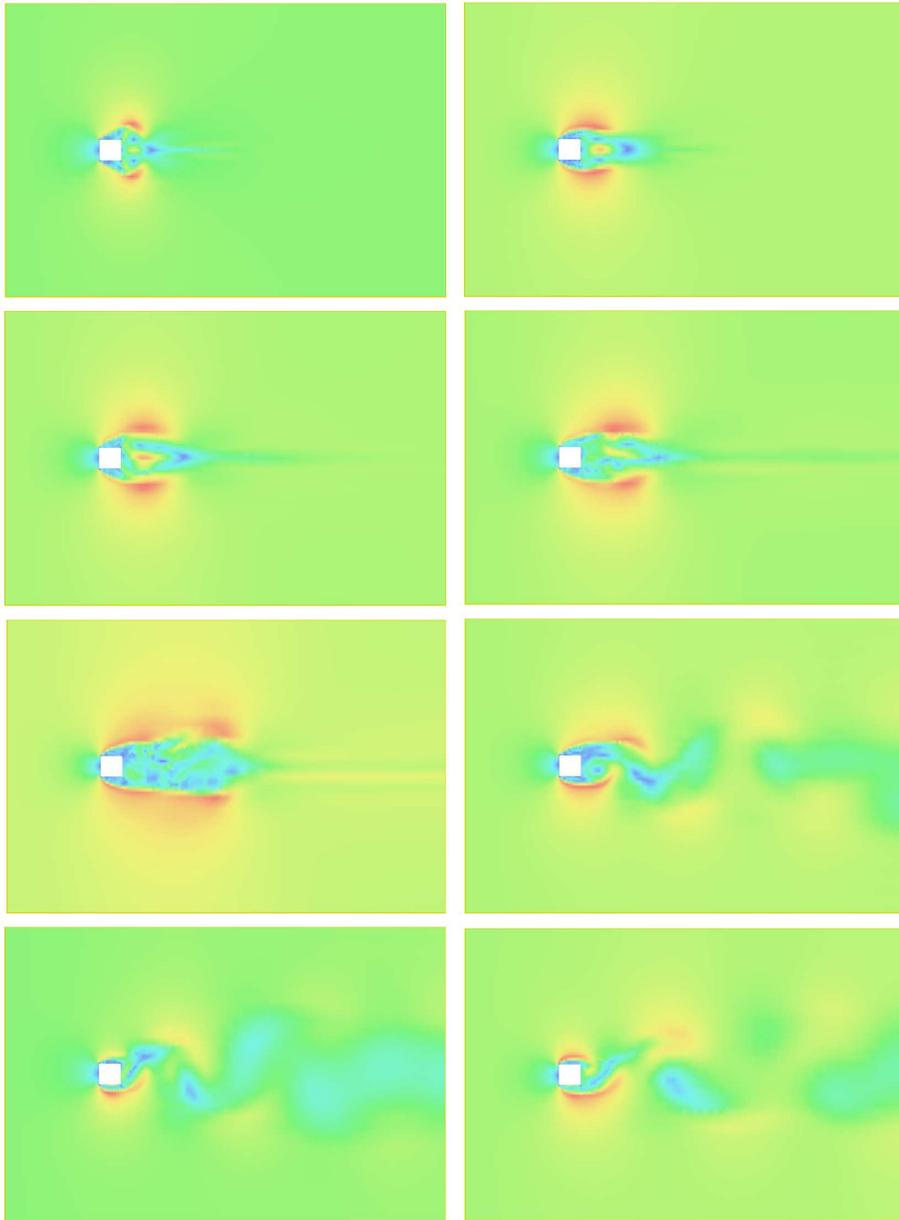
FIGURE 20.6. Magnitude of the computed velocity corresponding to zero initial data, for time steps 48,64,96,128,160,704,960,1024.
