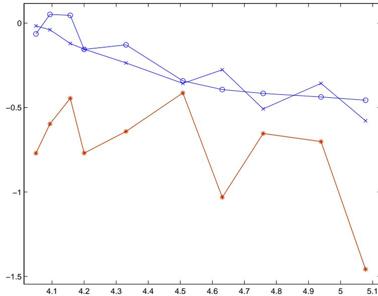
FIGURE 30.10. Square cylinder:  $\log_{10}$ - $\log_{10}$  plot of the a posteriori error estimates  $e_{D,h}$  ('o') and  $e_{M,h}$  ('x'), and the true error ('\*') based on  $c_D = 2.2$ , as functions of the number of mesh points in space.
