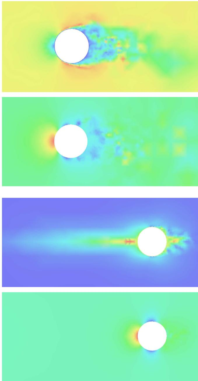
FIGURE 30.22. Sphere: magnitude of velocity and pressure (upper), and magnitude of dual velocity and pressure (lower).
