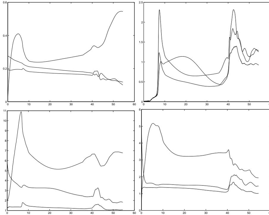
FIGURE 34.11.  $x_3$ -periodic Couette flow ( $\kappa\nu = 0.5$ ): Perturbations  $\|\varphi_i\|$  as functions of time (upper left), derivatives  $\|\partial u_i/\partial x_1\|$  (upper right),  $\|\partial u_i/\partial x_2\|$  (lower left), and  $\|\partial u_i/\partial x_3\|$  (lower right) as functions of time.
