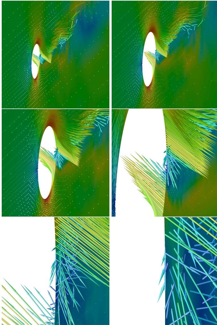
FIGURE 11.2. Snapshot of the velocity illustrating the single separation point.
