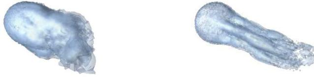
FIGURE 22.1. Vorticity for a sphere before (left) and after (right) drag crisis.
