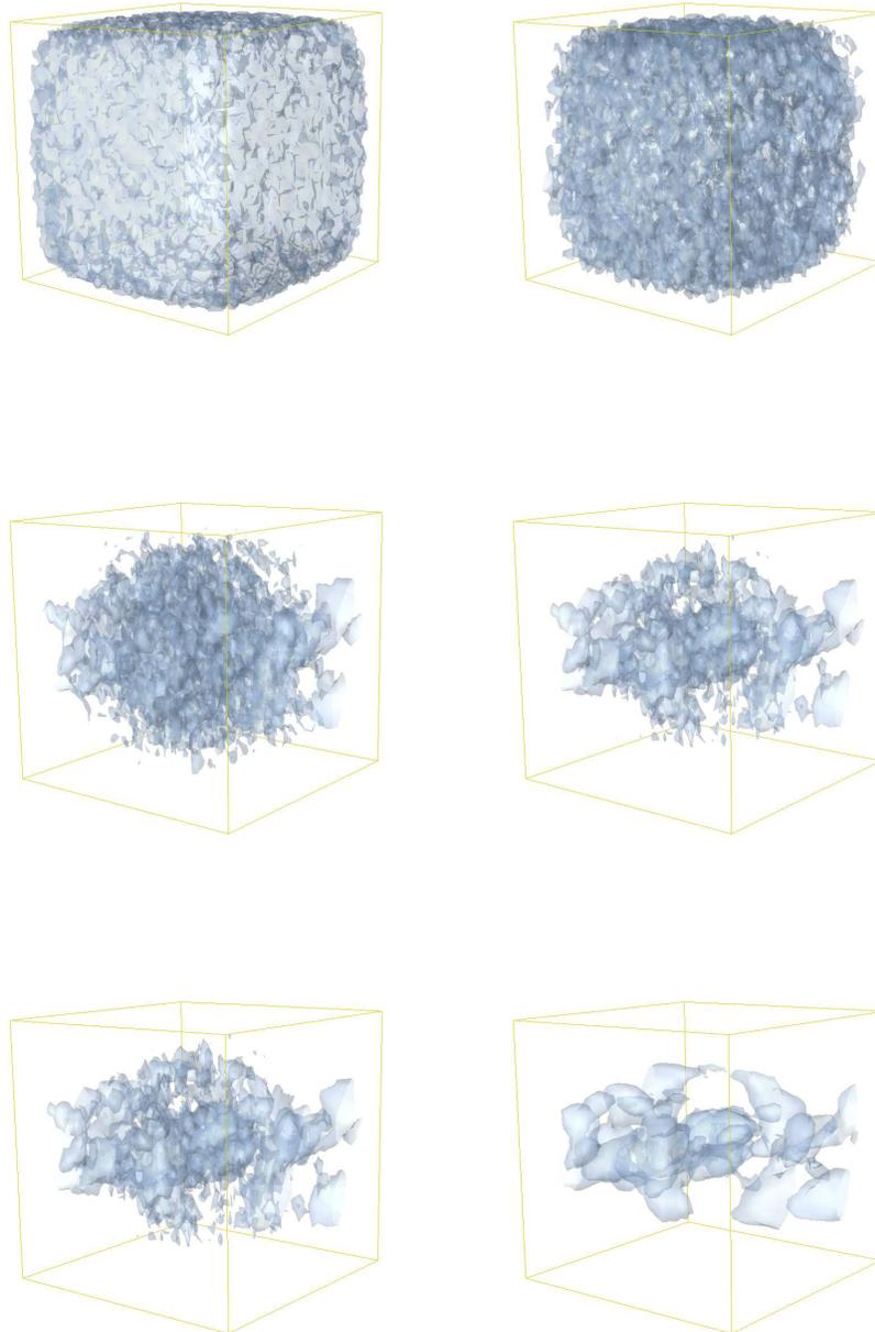
FIGURE 34.5. Streamwise velocity isosurfaces for  $|u_3| = 0.015$  in Couette flow (random initial perturbation) for  $t = 0, 1, 4, 5, 7, 10$
