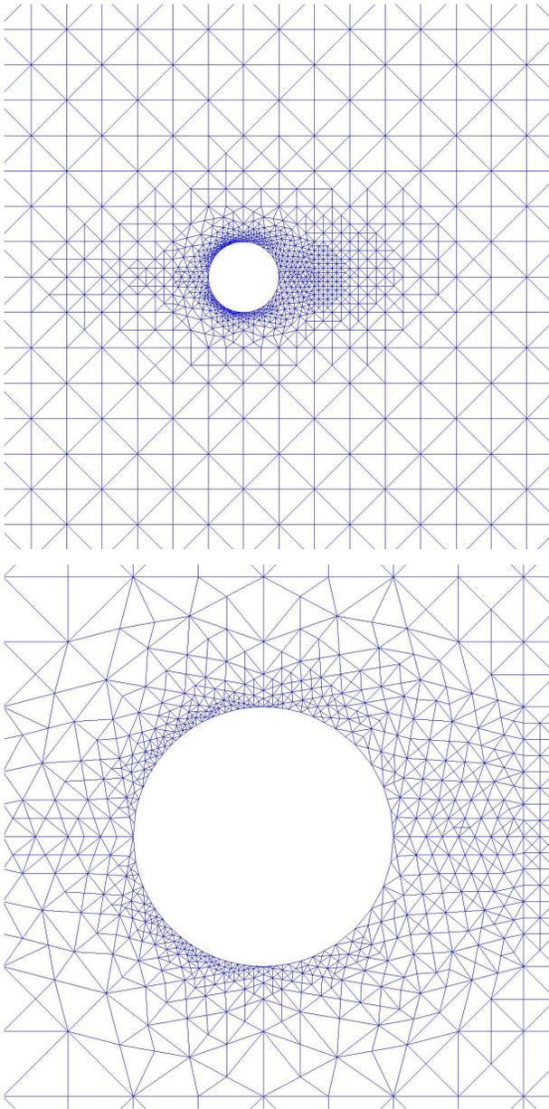
FIGURE 30.23. Sphere: computational mesh refined with respect to drag.
