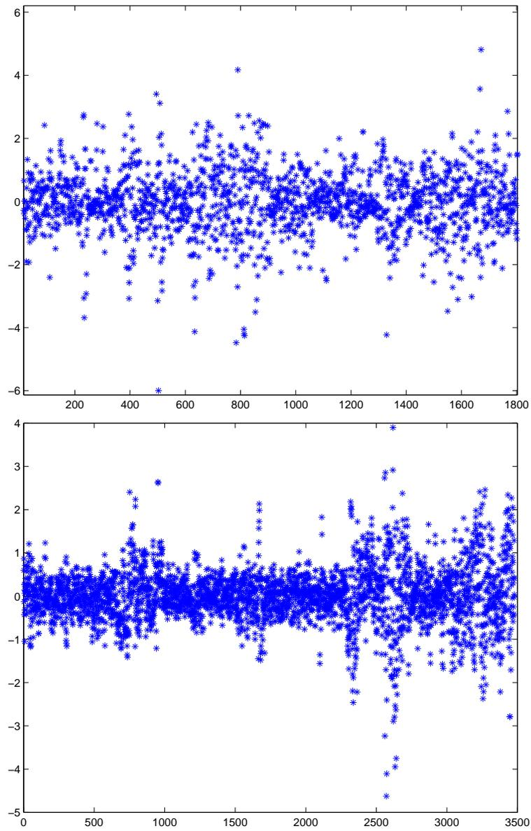
FIGURE 16.1. Sum of the real parts of the eigenvalues of  $\nabla U$ , for G2 solutions  $\hat{U}$  for a few thousand elements in the turbulent wake of a circular and a square cylinder, from computations presented in detail in Chapter 30.
