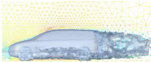
FIGURE 2.3. Turbulent flow around a car.
