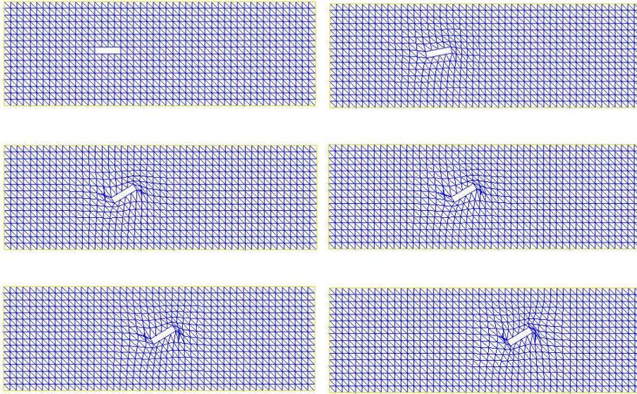
FIGURE 29.5. Mesh for moving  $0.25 \times 0.0625 \times 0.25$  object inside a channel.
