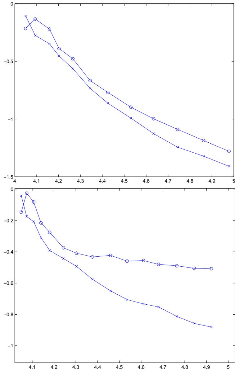
FIGURE 30.20. Circular cylinder: A posteriori error estimates  $e_D$  ('o')  $e_M$  ('x'), for  $Re = 100$  (upper) and  $Re = 3900$  (lower).
