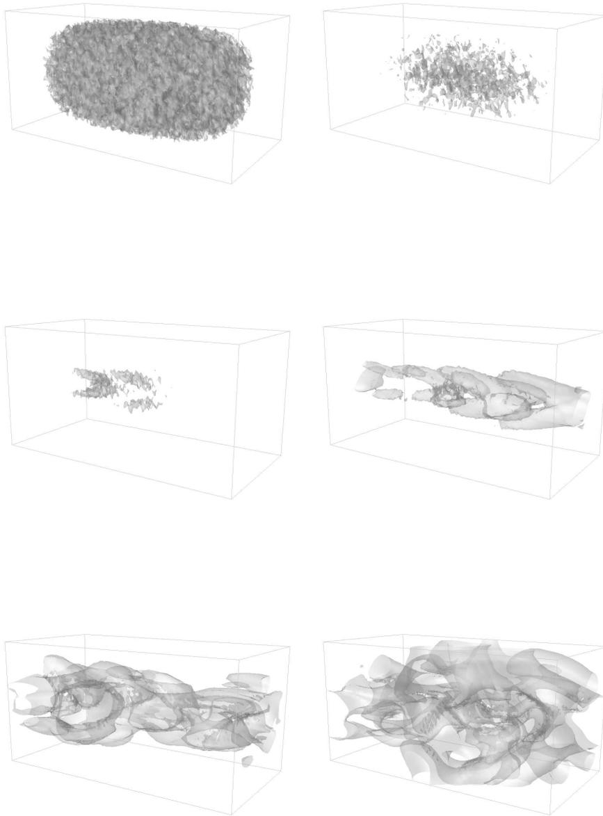
FIGURE 34.22. Transversal velocity isosurfaces for  $|u_3| = 0.02$  in jet flow (random initial perturbation) for  $t = 0, 2, 5, 7, 10, 15$
