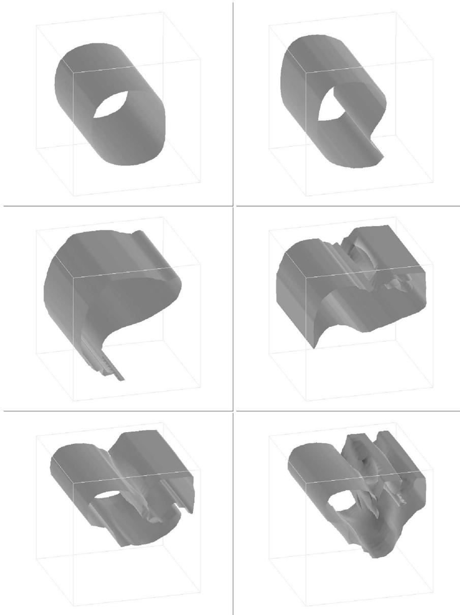
FIGURE 34.17. Velocity isosurfaces in Poiseuille flow ( $\kappa\nu = 0.1$ ) at  $t = 1, 3, \dots, 15$ , illustrating the Taylor-Görtler mechanism
