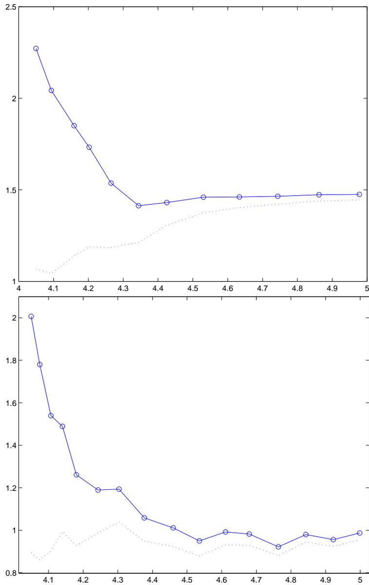
FIGURE 30.15. Circular cylinder: approximate drag coefficient as a function of the 10-logarithm of the number of mesh points in space, for  $Re = 100$  (upper) and  $Re = 3900$  (lower).
