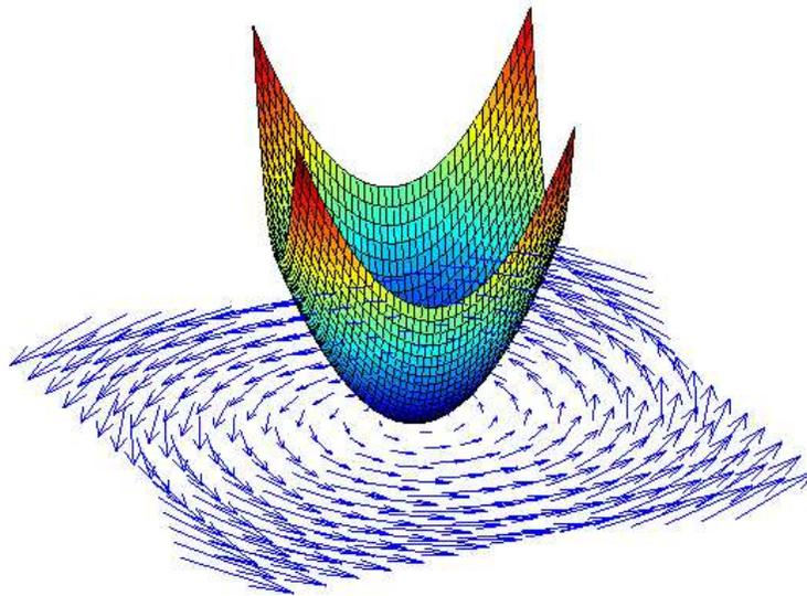
FIGURE 16.2. Rotational flow  $u(x) = \omega(-x_2, x_1, 0)$ , and  $p = \frac{\omega}{2}(x_1^2 + x_2^2)$ .
