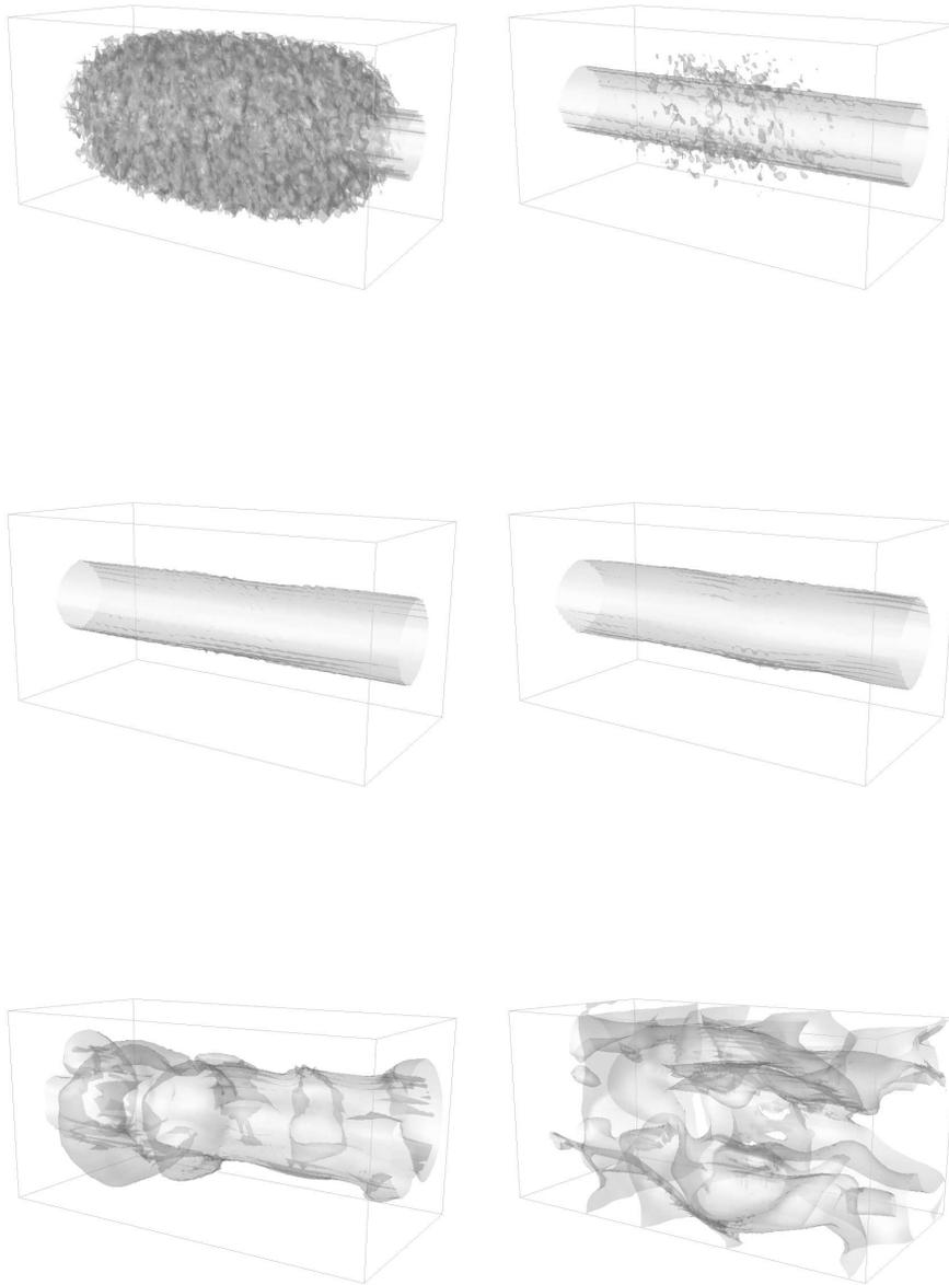
FIGURE 34.20. Streamwise velocity isosurfaces for  $|u_1| = 0.02$  in jet flow (random initial perturbation) for  $t = 0, 2, 5, 7, 10, 15$
