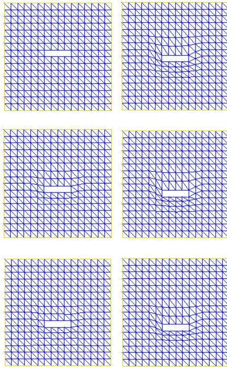
FIGURE 29.3. Box translation with Laplacian smoothing, for an  $0.25 \times 0.0625 \times 0.25$  object inside a  $0.5 \times 0.5625 \times 0.5$  box.
