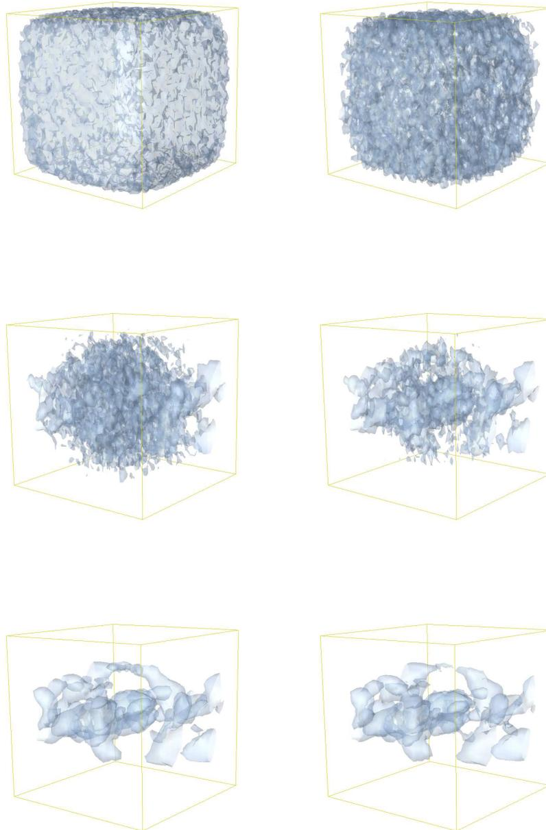
FIGURE 34.4. Streamwise velocity isosurfaces for  $|u_2| = 0.015$  in Couette flow (random initial perturbation) for  $t = 0, 1, 4, 5, 7, 10$
