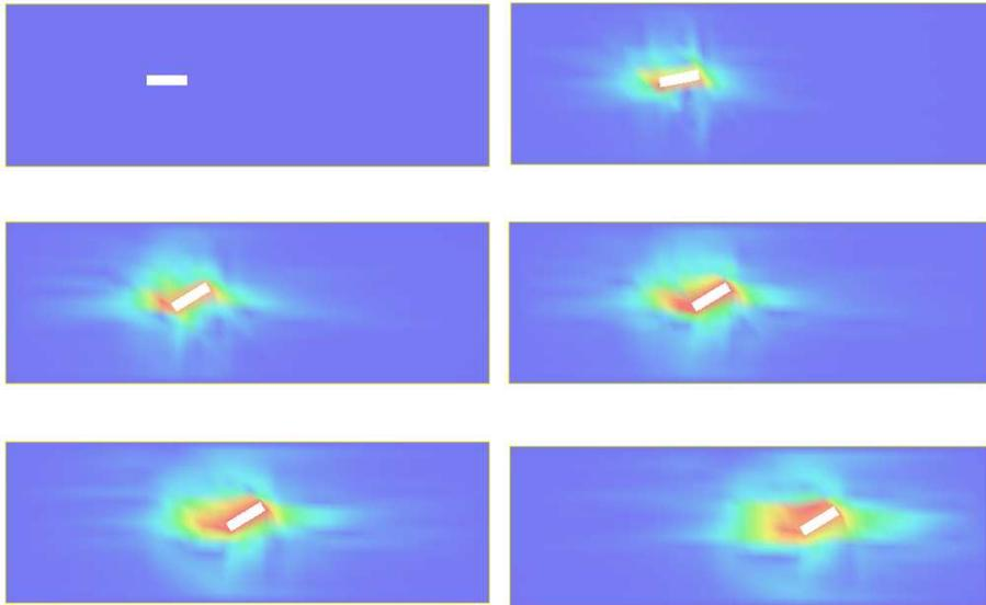
FIGURE 29.6. Magnitude of the velocity  $|u|$  for moving  $0.25 \times 0.0625 \times 0.25$  object inside a channel.
