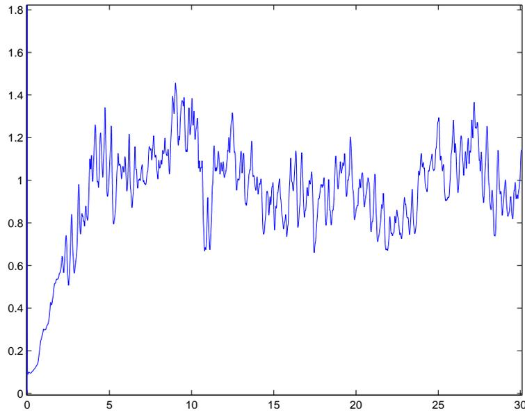
FIGURE 33.2. Time series of  $c_D$  for an EG2 solution.
