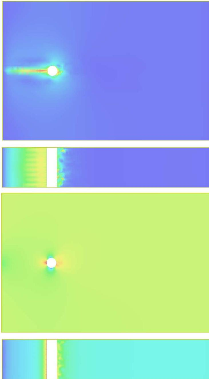
FIGURE 30.18. Circular cylinder at  $Re = 3900$ : magnitude of dual velocity  $|\varphi_h|$  (upper), and dual pressure  $|\theta_h|$  (lower).
