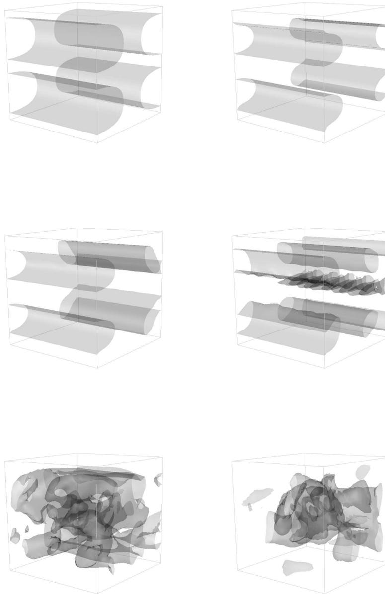
FIGURE 34.8. Transversal velocity isosurfaces for  $|u_2| = 0.2$  in Couette flow ( $\kappa\nu = 0.5$ ) for  $t = 0, 5, 10, 15, 20, 30$
