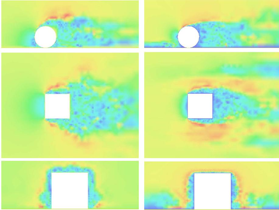
FIGURE 32.7. Snapshots of magnitude of velocity, for rotating (left) and stationary (right) cylinder, in the  $x_1x_2$ -,  $x_1x_3$ -, and  $x_2x_3$ -planes, through the center of the cylinder.
