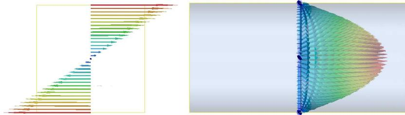
FIGURE 34.1. Couette flow (left) with a linear velocity profile, and Poiseuille flow (right) with a parabolic velocity profile.
