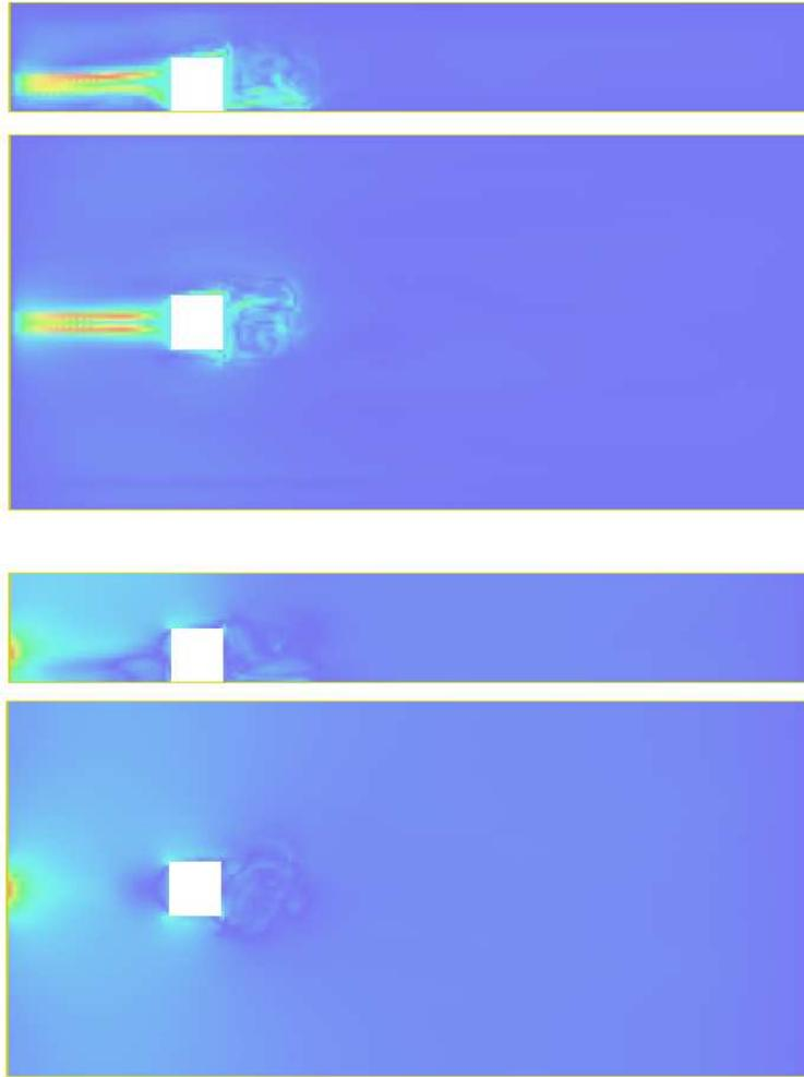
FIGURE 14.3. Surface mounted cube: dual velocity  $|\varphi_h|$  (upper), and dual pressure  $|\theta_h|$  (middle), in the  $x_1x_2$ -plane at  $x_3 = 3.5H$  and in the  $x_1x_3$ -plane at  $x_2 = 0.5H$ .
