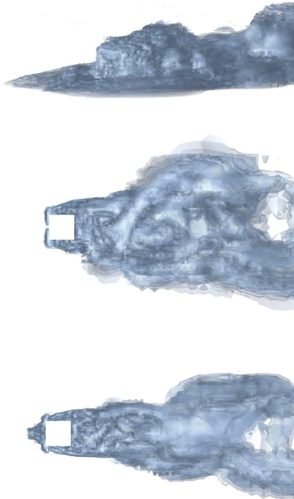
FIGURE 32.1. Isosurfaces for the magnitude of the vorticity for the cube (upper), the cylinder (middle), and the cylinder with a plate (lower).
