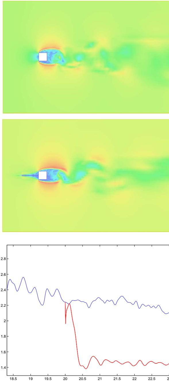
FIGURE 32.2. Magnitude of the velocity for the cylinder with and without the plate (upper), and a time series of the corresponding (normalized) drag forces when introducing the plate (lower).
