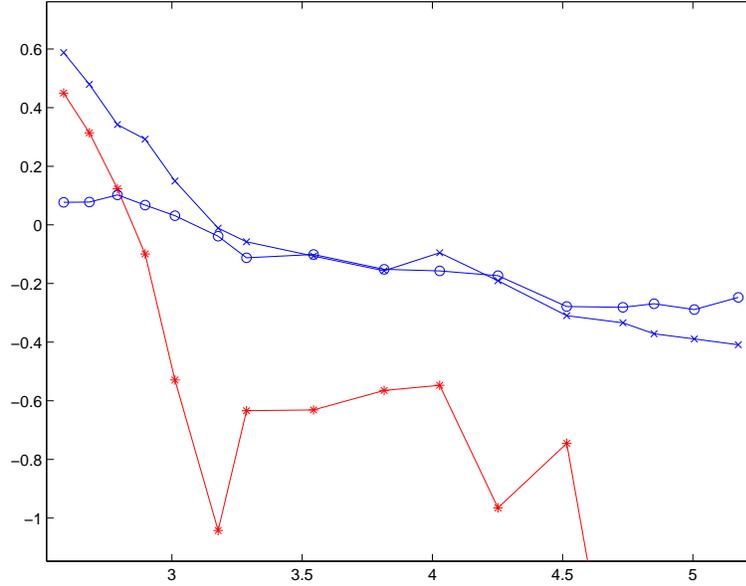
FIGURE 30.4. Surface mounted cube:  $\log_{10}$ - $\log_{10}$  plot of the a posteriori error estimates  $e_{D,h}$  ('o') and  $e_{M,h}$  ('x'), and the true error ('\*') based on  $c_D = 1.55$  (the solution on the finest mesh), as functions of the number of mesh points in space.
