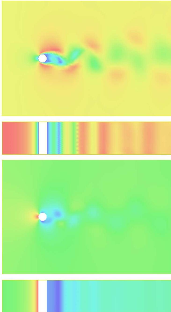
FIGURE 30.12. Circular cylinder at  $Re = 100$ : magnitude of velocity  $|U|$  (upper), and pressure  $P$  (lower).
