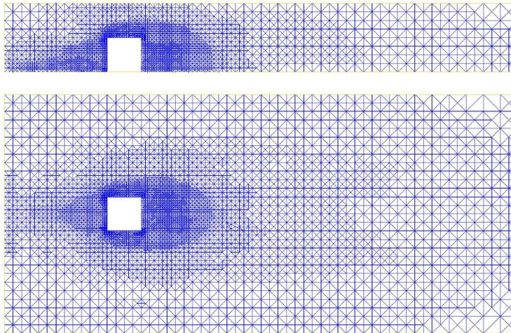
FIGURE 30.3. Surface mounted cube: computational mesh refined with respect to mean drag, in the  $x_1x_2$ -plane at  $x_3 = 3.5H$  and in the  $x_1x_3$ -plane at  $x_2 = 0.5H$ .
