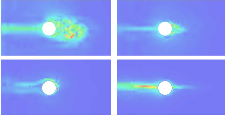
FIGURE 33.1. Magnitude of the dual velocity for  $\beta = 0.1$  (upper left),  $0.01$  (upper right),  $0$  (lower left), using velocity boundary data, and for  $\beta = 0$  using pressure data (lower right), in the  $x_1x_2$ -plane for  $x_3 = 0.2$ .
