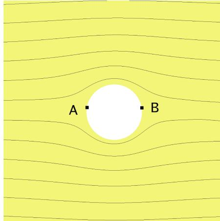
FIGURE 20.16. Streamlines for the potential solution of a circular cylinder.
