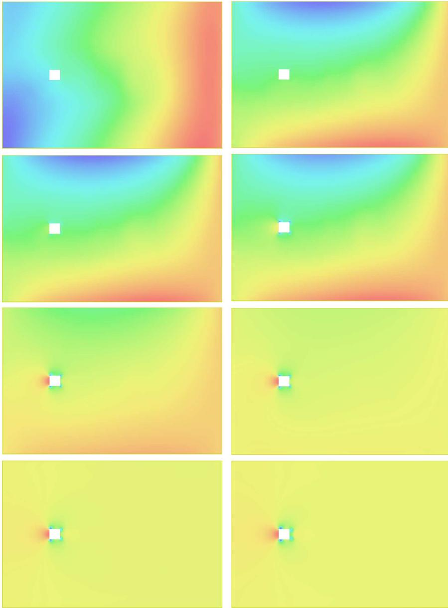
FIGURE 20.4. Computed pressure corresponding to the initial data  $U(0) = \nabla\phi$ , for time steps no 1,2,4,5,6,7,20,37.
