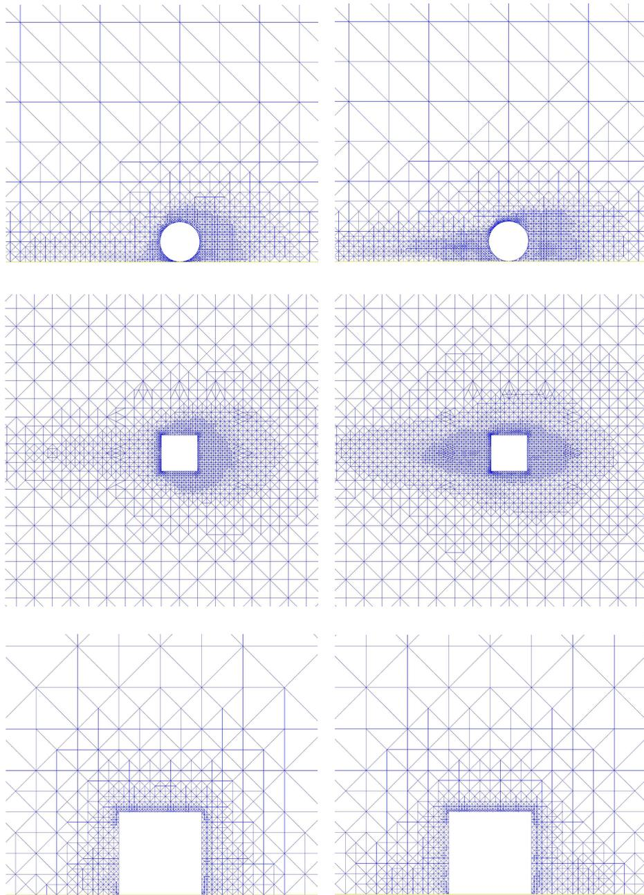
FIGURE 32.9. Refined mesh for the rotating (left) and the stationary (right) cylinder, in the  $x_1x_2$ -,  $x_1x_3$ -, and  $x_2x_3$ -planes.
