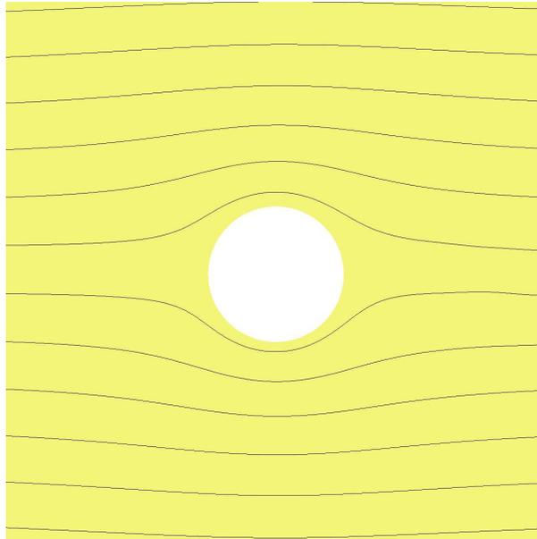
FIGURE 8.3. Streamlines for the potential solution of a circular cylinder.
