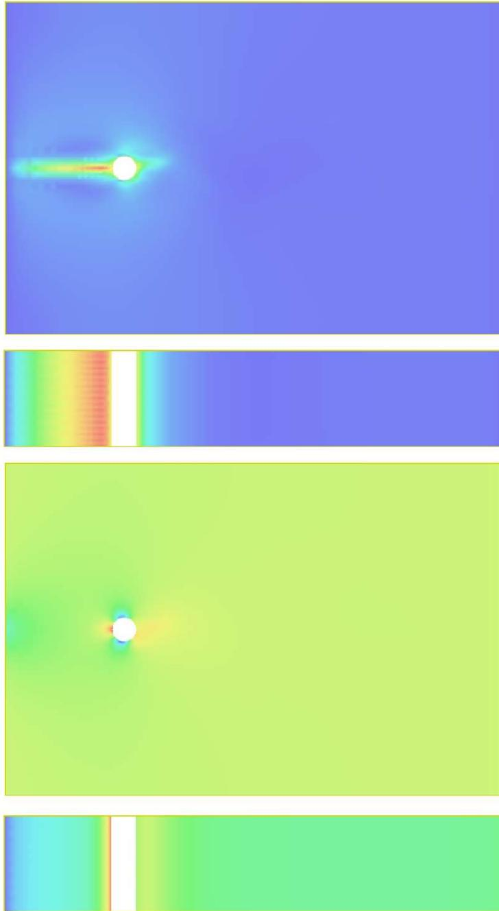
FIGURE 30.17. Circular cylinder at  $Re = 100$ : magnitude of dual velocity  $|\varphi_h|$  (upper), and dual pressure  $|\theta_h|$  (lower).
