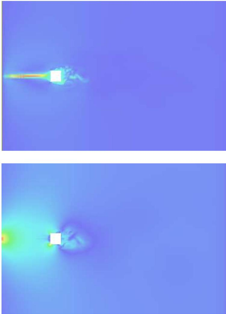
FIGURE 30.8. Square cylinder: dual velocity  $|\varphi_h|$  (upper), and dual pressure  $|\theta_h|$  (lower), in the  $x_1x_3$ -plane at  $x_2 = 7D$  and in the  $x_1x_2$ -plane at  $x_3 = 2D$ .
