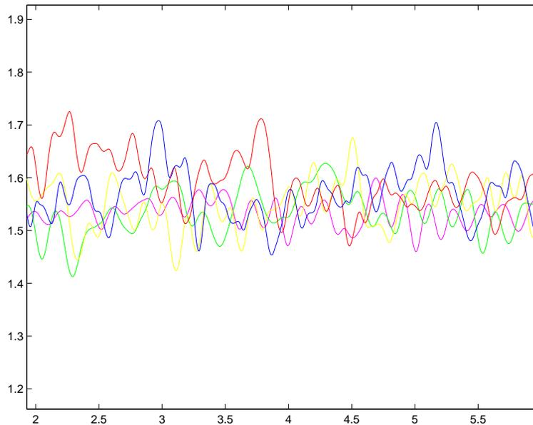
FIGURE 14.1. Drag  $D(t)$  (normalized) for a surface mounted cube, as a function of time, for 5 computational meshes.
