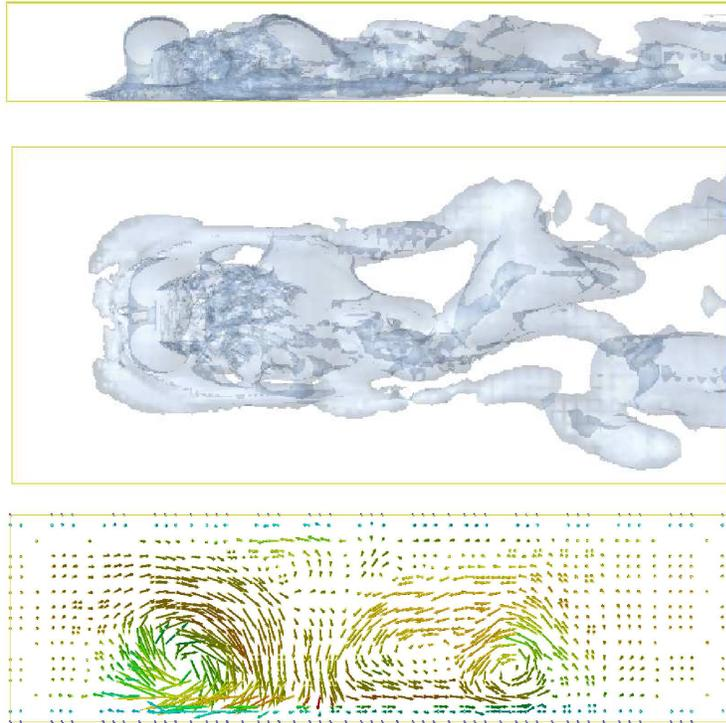
FIGURE 34.18. Surface mounted cube: isosurfaces for  $|(u_2, u_3)|$  in the  $x_1x_2$ -plane (upper), in the  $x_1x_3$ -plane (middle), and the velocity field in the  $x_2x_3$ -plane downstream the cube (lower).
