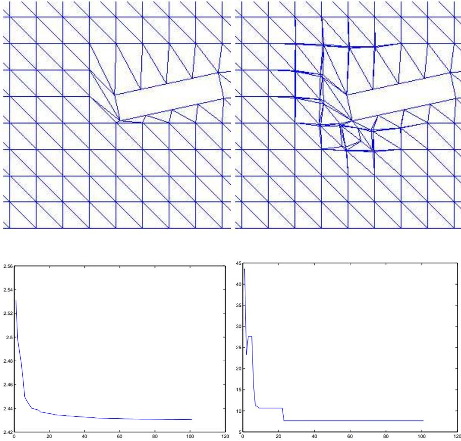
FIGURE 29.1. Locally distorted mesh before (upper left) and after (upper right), 100 iterations of the local optimization algorithm. The weighted  $l_2$ -norm (lower left) and the max-norm (lower right), of the square root of the condition numbers of  $A^T A$  as functions of number of iterations.
