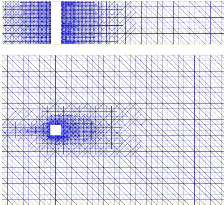
FIGURE 30.9. Square cylinder: computational mesh after 9 adaptive mesh refinements with respect to mean drag, in the  $x_1x_3$ -plane at  $x_2 = 7D$  and in the  $x_1x_2$ -plane at  $x_3 = 2D$ .
