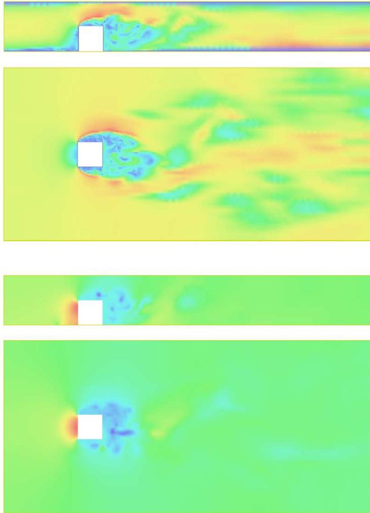
FIGURE 14.2. Surface mounted cube: velocity  $|U|$  (upper) and pressure  $P$  (lower), in the  $x_1x_2$ -plane at  $x_3 = 3.5H$  and in the  $x_1x_3$ -plane at  $x_2 = 0.5H$ .
