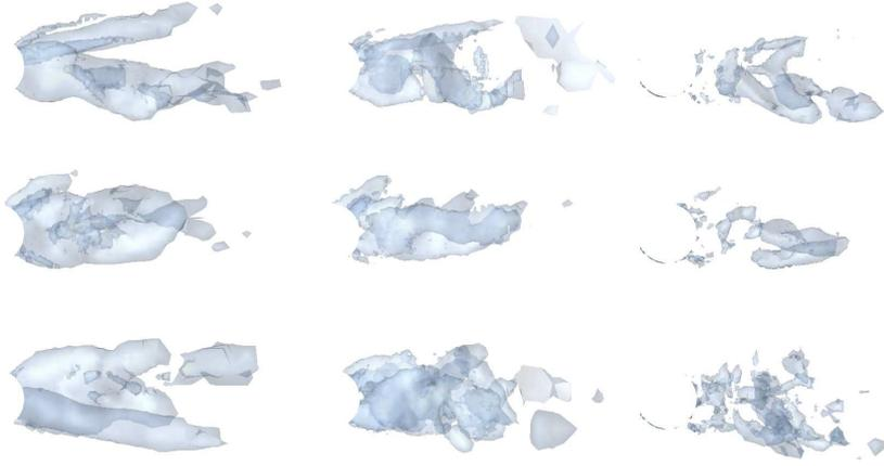
FIGURE 11.3. Isosurfaces for vorticity  $\omega = (\omega_1, \omega_2, \omega_3)$ :  $\omega_1$  (left),  $\omega_2$  (middle), and  $\omega_3$  (right), at three times  $t_1 < t_2 < t_3$  (upper, middle, lower), in the  $x_1x_2$ -plane.
