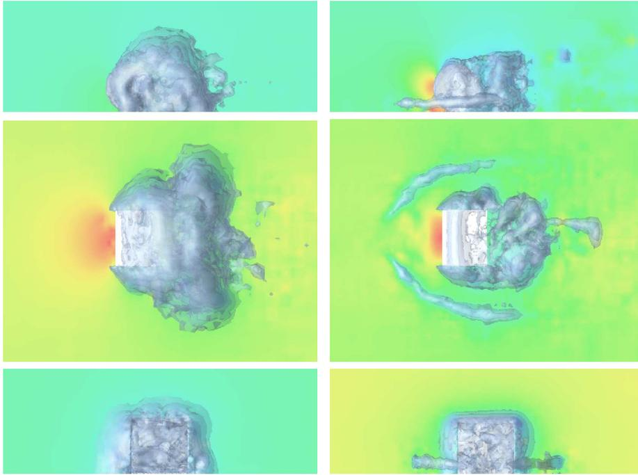
FIGURE 32.8. Snapshots of pressure and isosurfaces of negative pressure, for rotating (left) and stationary (right) cylinder, in the  $x_1x_2$ -,  $x_1x_3$ -, and  $x_2x_3$ -planes, through the center of the cylinder.
