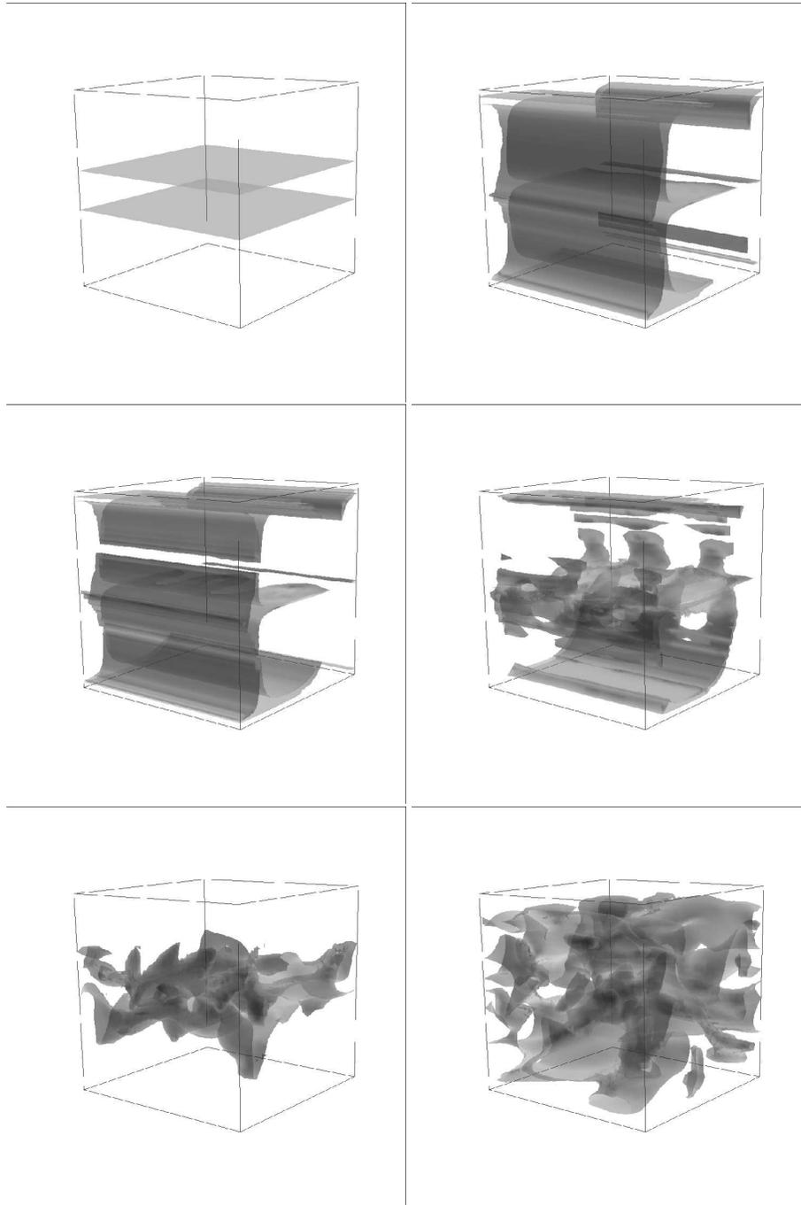
FIGURE 34.13. Streamwise velocity isosurfaces for  $|u_1| = 0.2$  in  $x_3$ -periodic Couette flow ( $\kappa\nu = 0.5$ , random force perturbation) for  $t = 0, 5, 6, 7, 10, 20$
