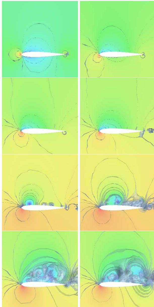
FIGURE 23.1. Simulation of take-off for a 3d wing using Euler/G2, with increasing angle of attack from 0 to 17 degrees.
