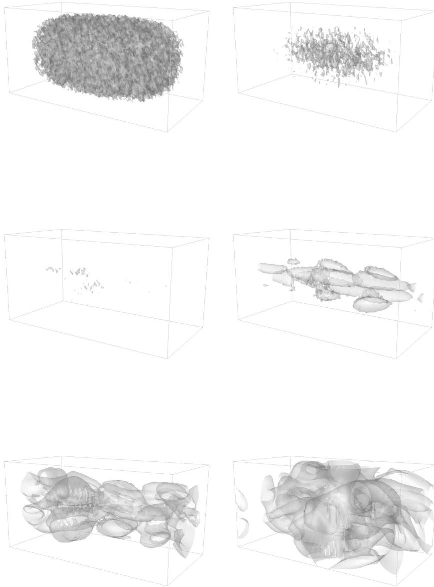
FIGURE 34.21. Transversal velocity isosurfaces for  $|u_2| = 0.02$  in jet flow (random initial perturbation) for  $t = 0, 2, 5, 7, 10, 15$
