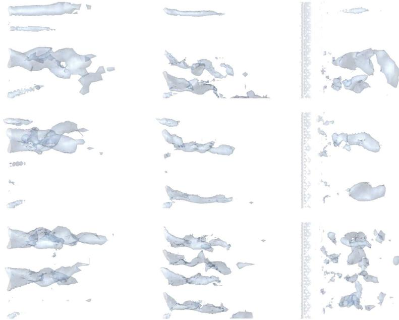
FIGURE 11.4. Isosurfaces for vorticity  $\omega = (\omega_1, \omega_2, \omega_3)$ :  $\omega_1$  (left),  $\omega_2$  (middle), and  $\omega_3$  (right), at three times  $t_1 < t_2 < t_3$  (upper, middle, lower), in the  $x_1x_3$ -plane.
