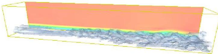
FIGURE 31.1. Transition to turbulence in a boundary layer computation, introducing Taylor-Görtler type perturbations (see Chapter 34) of amplitude 0.1 at the inflow.
