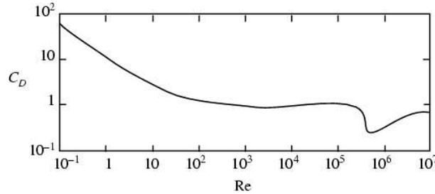
FIGURE 32.3.  $c_D$  for a circular cylinder as a function of Reynolds number.
