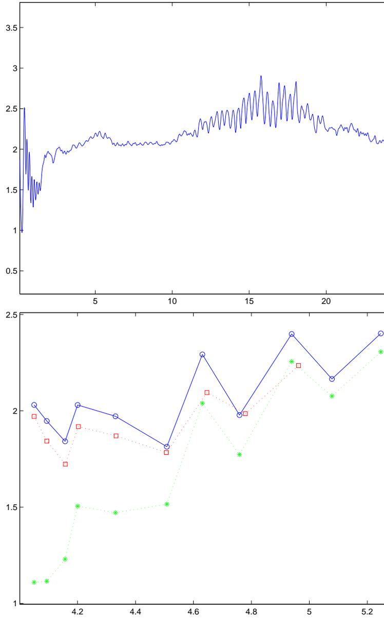
FIGURE 30.7. Square cylinder: Normalized drag force as a function of time after 9 mesh refinements (upper), and  $\bar{c}_D^h$  ('o'), the corresponding approximations without the contribution from the stabilizing term in (30.3) (\*), and the approximation with 2% white noise in inflow velocity ('□'), as functions of the 10-logarithm of the number of mesh points in space (lower).
