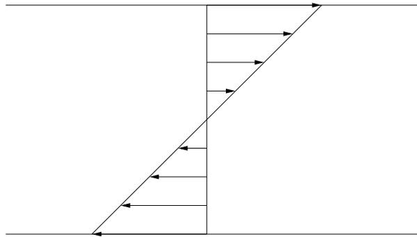
FIGURE 8.4. Couette flow: parallel shear flow.
