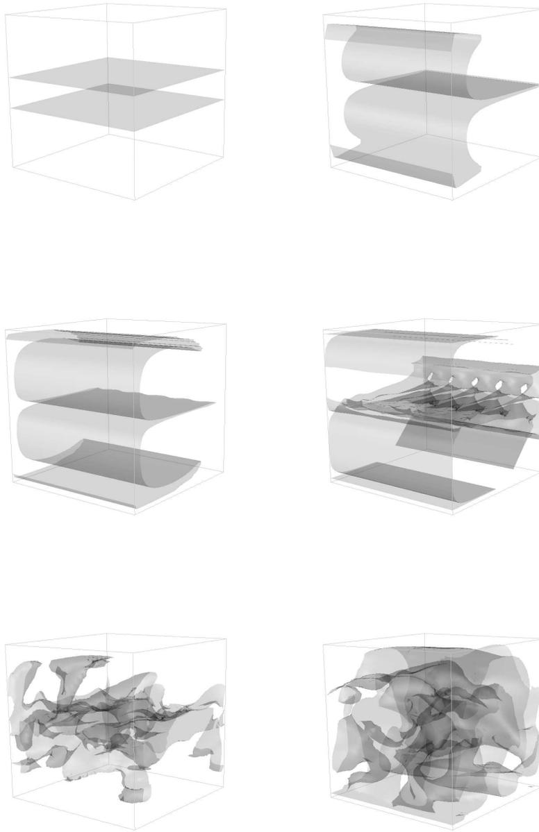
FIGURE 34.7. Streamwise velocity isosurfaces for  $|u_1| = 0.2$  in Couette flow ( $\kappa\nu = 0.5$ ) for  $t = 0, 5, 10, 15, 20, 30$
