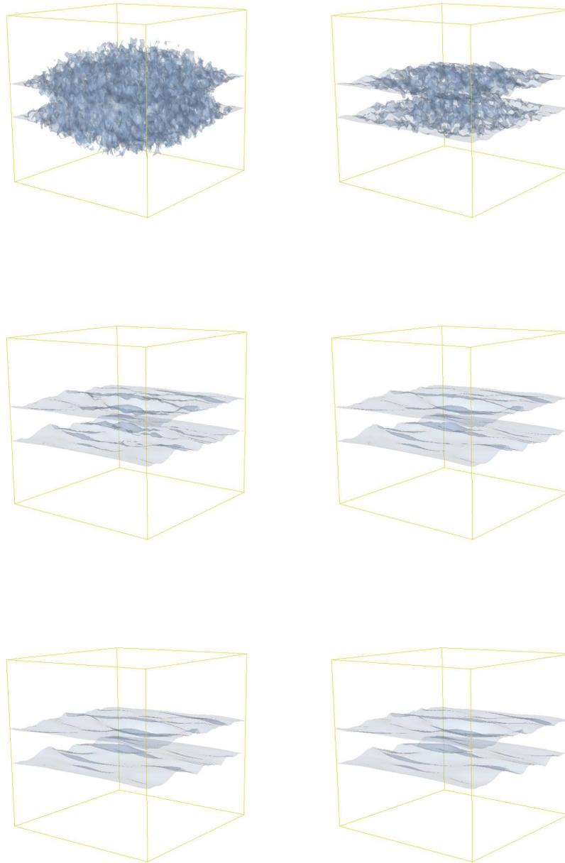
FIGURE 34.3. Streamwise velocity isosurfaces for  $|u_1| = 0.2$  in Couette flow (random initial perturbation) for  $t = 0, 1, 4, 5, 7, 10$
