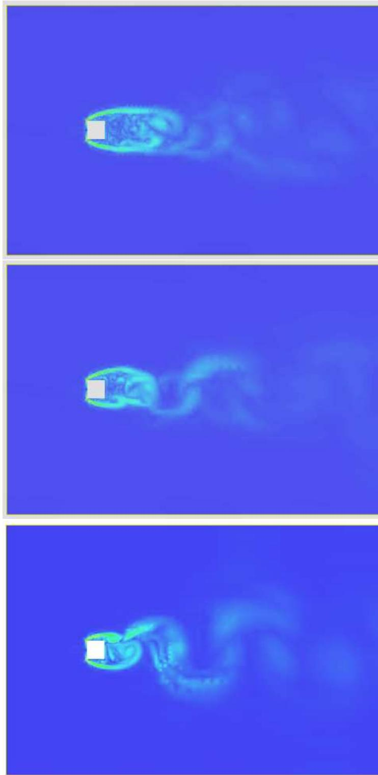
FIGURE 30.6. Time evolution of vorticity  $|\nabla \times U|$ , in the  $x_1x_2$ -plane at  $x_3 = 2D$ .
