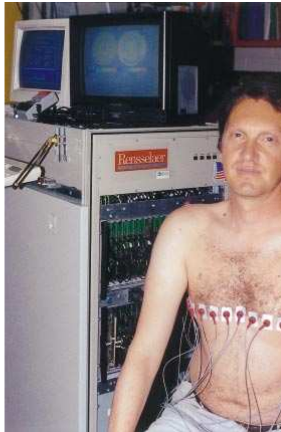
Fig. 3 The ACT 3 system with 32 electrodes encircling the chest of a subject. Here the goal is to make images that show the changes in volumes of air and blood that occur with breathing and the pulsatile circulation of the blood. Such images are referred to as ventilation and perfusion images, respectively. This is one possible positioning of electrodes for this purpose.
