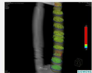
Figure 4: 4D PC-MRI measurement of a prototypic aortic phantom.
