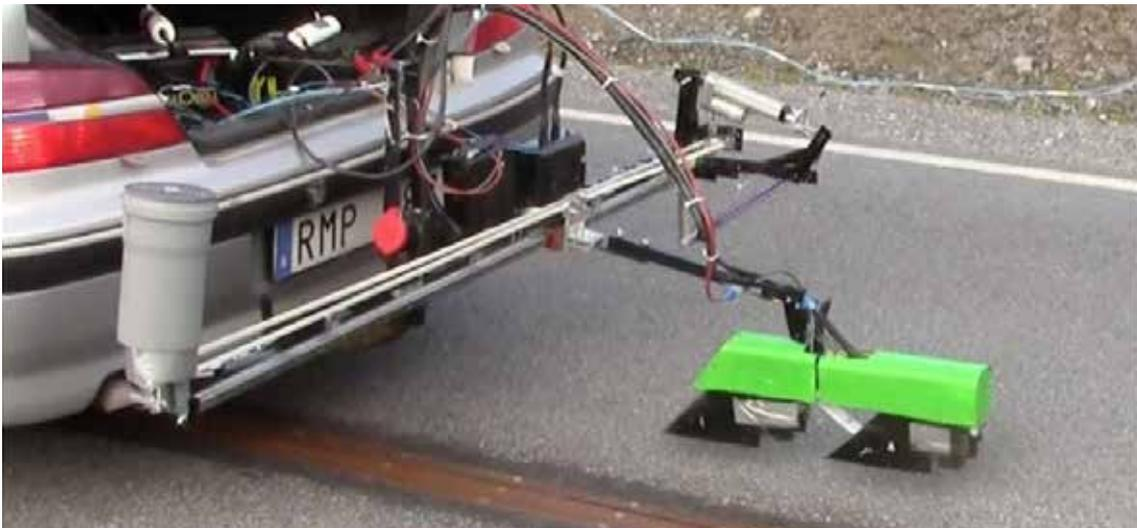
Figure 4-13 Power-take-off unit with position control from a student project at Chalmers [31]
