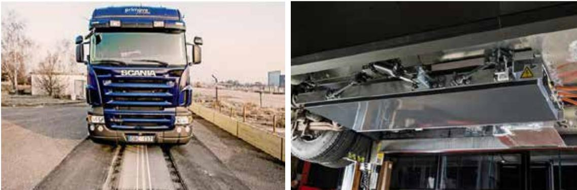
**Figure 8-5** Picture of test vehicle operating on the 800 m track for demonstrating Bombardiers concept for dynamic inductive power transfer, and picture of the receiving-side coil when installed on the vehicle [54]
