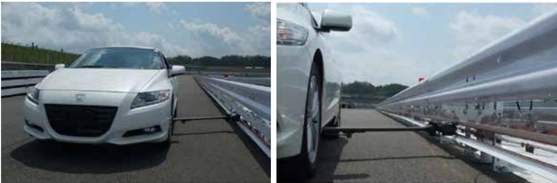
Figure 5-1 Pictures of dynamic charging system developed by Honda when installed on an electric vehicle in operation on a test track [34], [35]
