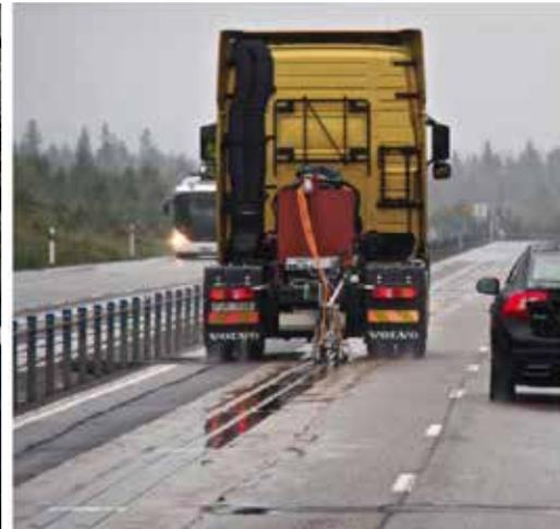
**Figure 4-1 APS power supply systems from Alstom for tram and truck applications**
