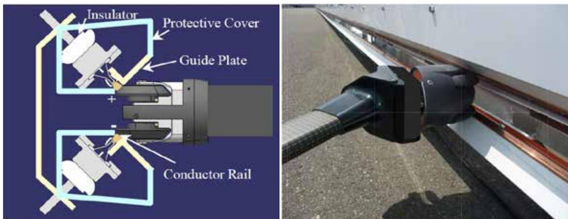
**Figure 5-3** Illustration of two-phase sliding for power supply from the side of the road, [34], and closer picture of the power take-off unit when in operation [33]
