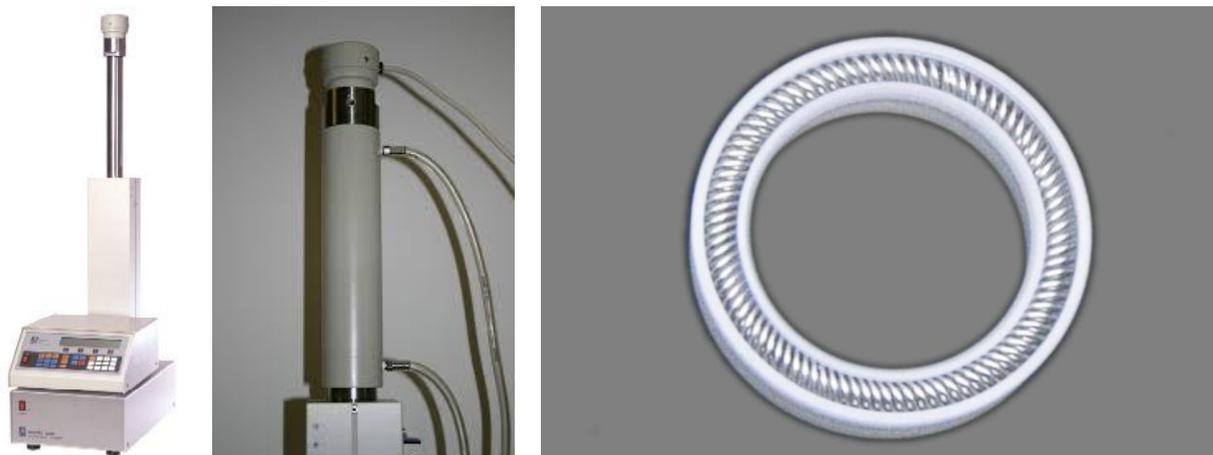
Figure 2.5: High pressure syringe pump. Left, pump and control modules; Middle, thermostatic jacket fitted to pump cylinder; Right, piston sealing ring.
