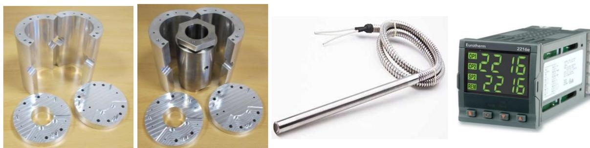
Figure 2.3: From left to right: photographs of the heating jacket components; heating jacket components with view cell; electric cartridge heater; and process controller.
