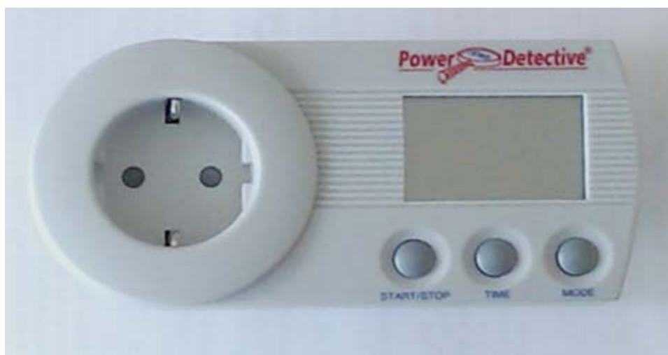
Figure 5.1 Power Detective - plug for metering of end-use demand
