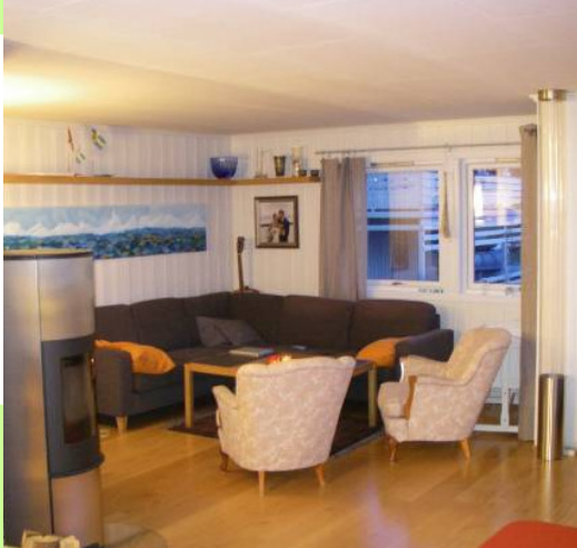
Living room after renovation. The transparent ventilation duct to the right provides fresh air to the office and one of the bedrooms in the base floor. A 5W LED lamp is installed within.
