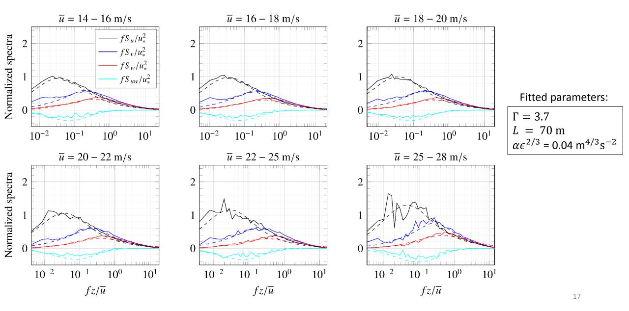
Measured vs NORSOK vs IEC Kaimal spectra
