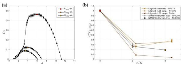
Figure 3 (a)  $C_p$ - $\lambda$ -curves of the three aligned turbines, all referred to  $u_{\text{ref}}=11.5$  m/s
