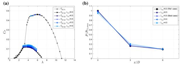
Figure 4 (a)  $C_p$ - $\lambda$ -curves of the second turbine T2 depending on different tip speed ratios of T1
