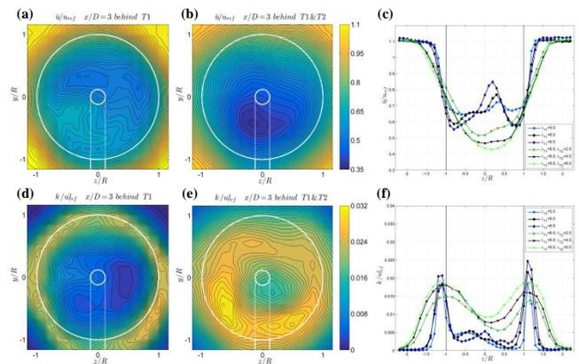
Figure 6 (a,b,c) Normalized mean velocity and (d,e,f) Normalized turbulent kinetic energy
