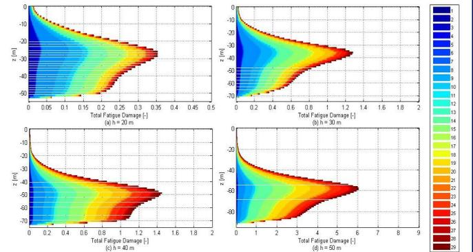
Figure 4: Total fatigue damage, showing contributions from each environmental condition.
