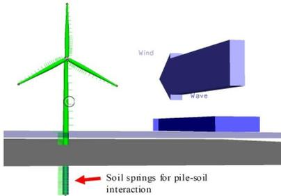
Figure 2: DTU 10 MW model in RIFLEX
