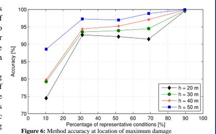
Figure 6: Method accuracy at location of maximum damage
