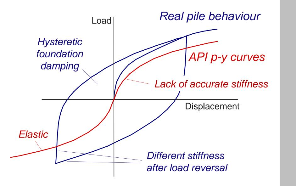
Their applicability to predict pile behaviour in integrated analyses of OWT has been questioned, and new foundation models are needed.
