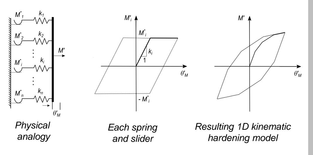
The model is composed of a rigid element connecting mudline with the plastic decoupling point, an elastic stiffness matrix and a 1D kinematic hardening model
