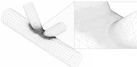
**44 FEM simulations** are run to compare both kind of meshing. SCF is computed at the brace toe position.
