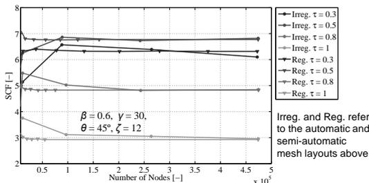
Convergence of the solution to a constant value for increasing number of nodes is clear for the semi-automatic mesh models. An asymptotic tendency is not obtained for the automatic mesh models for all cases until a great refinement is set. Solutions between both kind of models match for increasing mesh density. This grants the irregular mesh model reliability for a dense enough mesh.
