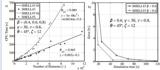
An error of less than 1% for SHELL93 is found for an element size of  $t_1 \times t_1$  and  $t_{CPU} = 35$  s. Same precision requires around 55 s for SHELL43.
