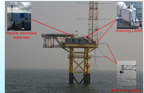
Meteorological OBLO instrumentation deployed at the German research platform FINO1 in the North Sea.
