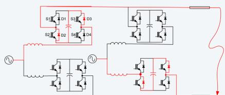
Figure: Full bridge MMC DC fault response
