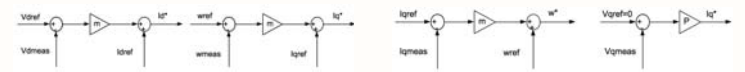
Figure 3: Conventional solution: P/V and Q/f droop | Our solution: P/V and f/Q droop
