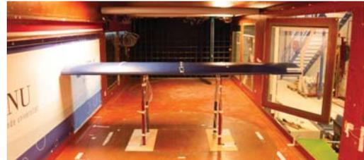
The lift and drag of the wing was measured for different angle of attack, for both clean condition (at turbulence intensities) and with applied roughness of different size and at different position at the leading edge.
