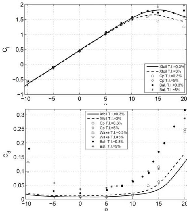
**Effect of roughness.** Lift and drag coefficients in function of angle of attack for  $Re=8.7 \cdot 10^5$  obtained with the balance. Grains (size  $\approx 0.5mm$ ) applied on the suction side between 4% and 7% of the chord ( $x/c$  4-7%). Tape applied around the leading edge between 0.9% on the suction side and 3.8% on the pressure side (LETape  $x/c$  0.9%t-3.8%b). Grains applied around the leading edge between 7.4% on the suction side and 7.9% on the pressure side ( $x/c$  7.4%t-7.9%b).
