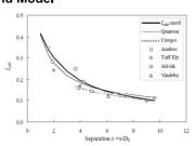
Added Turbulence Intensity versus turbine position By different model and wind farm measurements [2]
