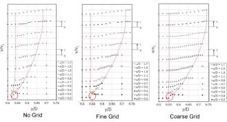
Downwind velocity distribution normalized by the design oncoming wind velocity of v1=12 m/s x/D is the axial downwind distance normalized by the wind turbine diameter y/D is the radial distance normalized by the wind turbine diameter
