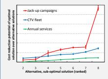
Jack-up vessel decisions have high potential for cost reduction but are associated with high uncertainties (failures requiring jack-up vessels happen rarely but each failure has large cost implications)
