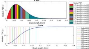
The values gained were used as deterministic values in combination with stochastic  $a_0/c_0$  ratio of initial crack sizes for the probabilistic reliability models.
