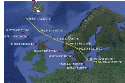
Figure 6. Mean sea level pressure in hPa (yellow) and maximum wind power density in \text{W/m}^2 at 100 m (red) tracks for cyclone Xaver as simulated by WRF model.
