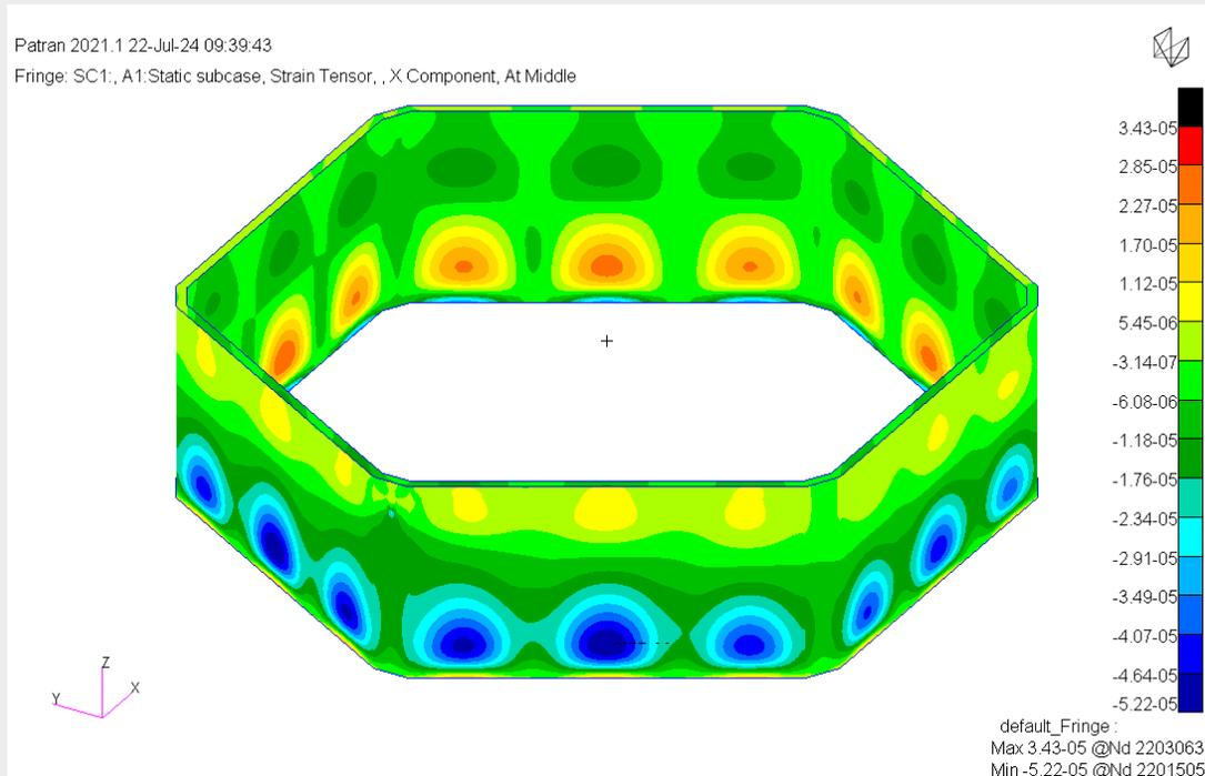
Vertical strain, outer perimeter wall. DLC6.1 Max\_HydroMy
