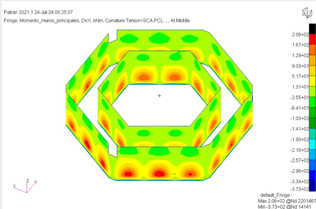
Bending moment [kNm], horizontal direction, perimeter walls. DLC6.1\_Max\_HydroMy
