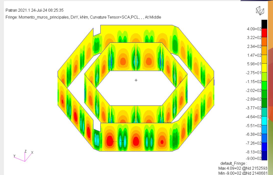
Bending moment [kNm], vertical direction, perimeter walls. DLC6.1\_Max\_HydroMy
