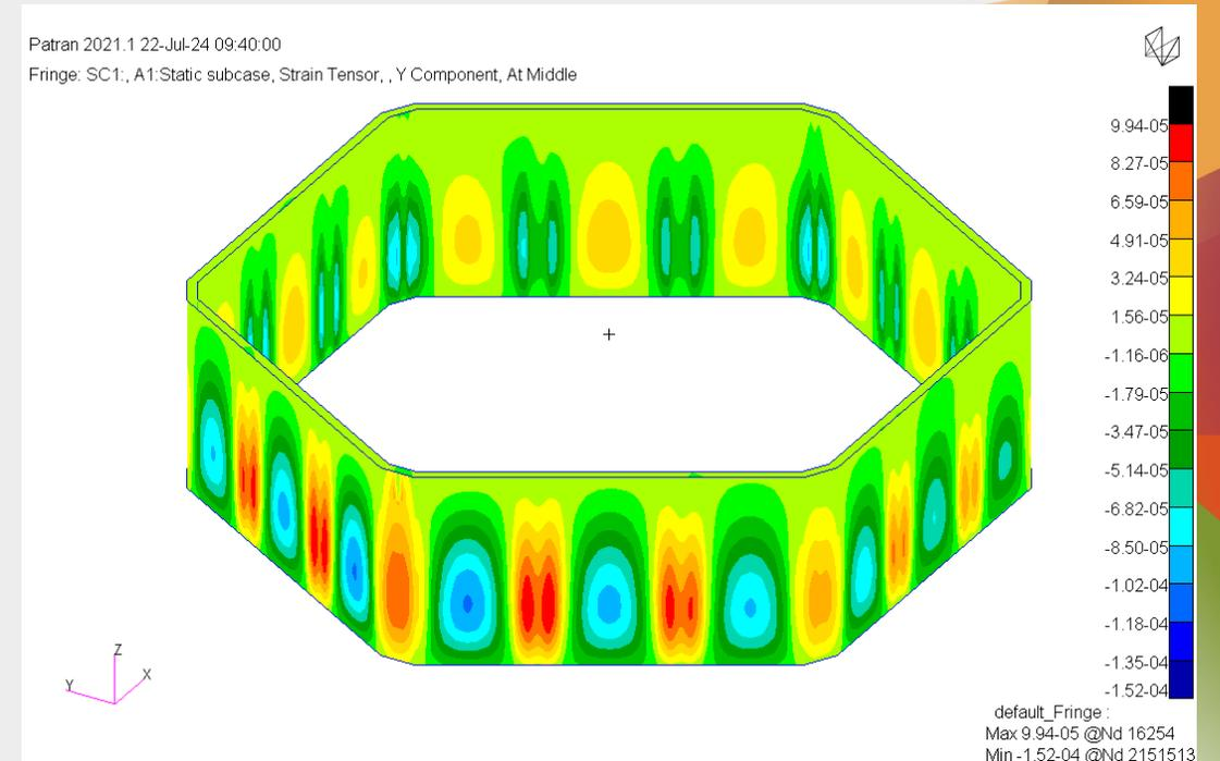
Horizontal strain, outer perimeter wall. DLC6.1 Max\_HydroMy
