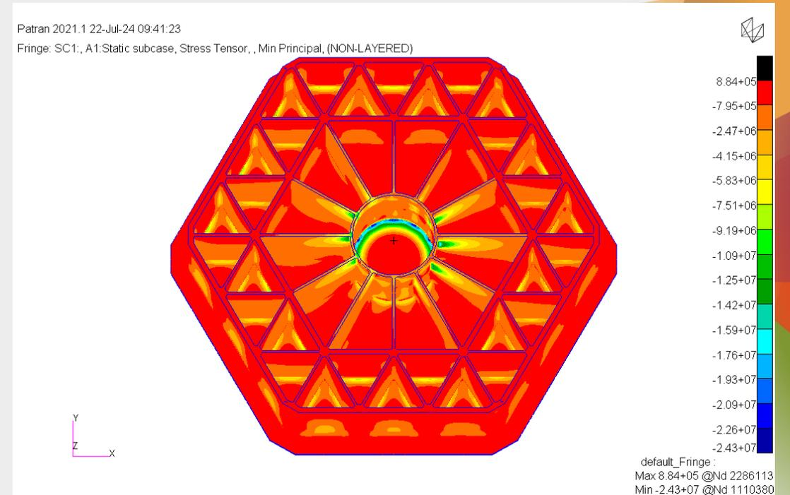
Minimum principal stress [Pa], concrete. DLC6.1 Max\_ HydroMy
