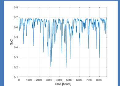
SoC of 50MWh battery - single turbine - 60s time constant
