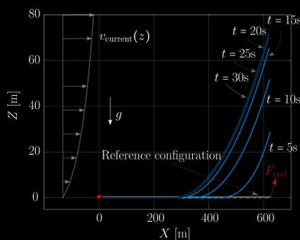
Figure 1: Snapshots of the studied mooring line, computed with cubic  $C^1$  isogeometric discretization.
