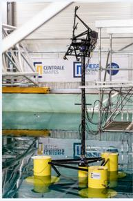
A model of the NREL-5MW wind turbine on the OC4 Semi-Submersible platform [1] was tested in the ECN wave-tank. The goal was to investigate the behaviour of various controllers in realistic conditions, not always well captured by numerical simulations. A software-in-the-loop method was used, using OpenFAST to compute the aerodynamic loads that are applied on the model via an actuator.
