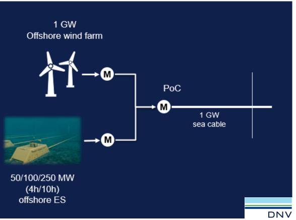
Following analysis, it was found that a 4h system with 50 – 100MW capacity is the optimum solution for the given market and the project concept.
