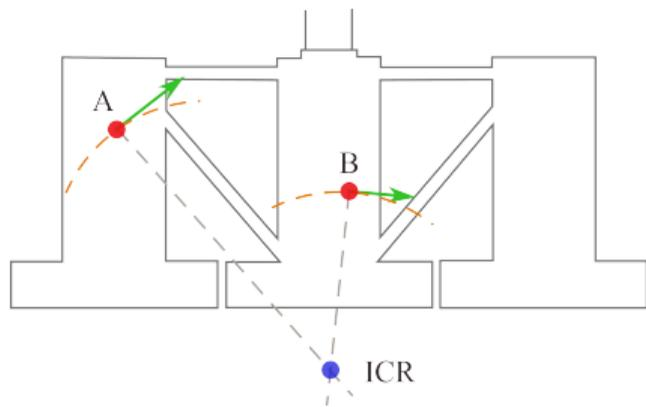
**Figure:** Construction of ICR
