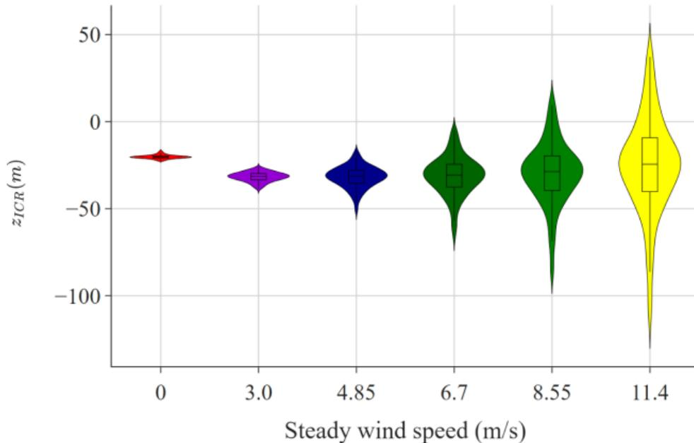
**Figure:** The ICR of FOWT in regular waves and steady wind - distribution of z coordinate
