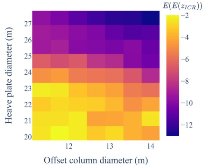
**Figure:** Design space - OC4 semi. Smaller members lead to higher  $z_{ICR}$
