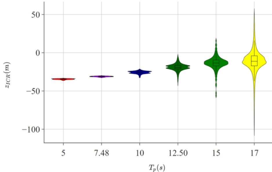
**Figure:** The ICR of FOWT simulated in regular waves - distribution of  $z$  coordinate
