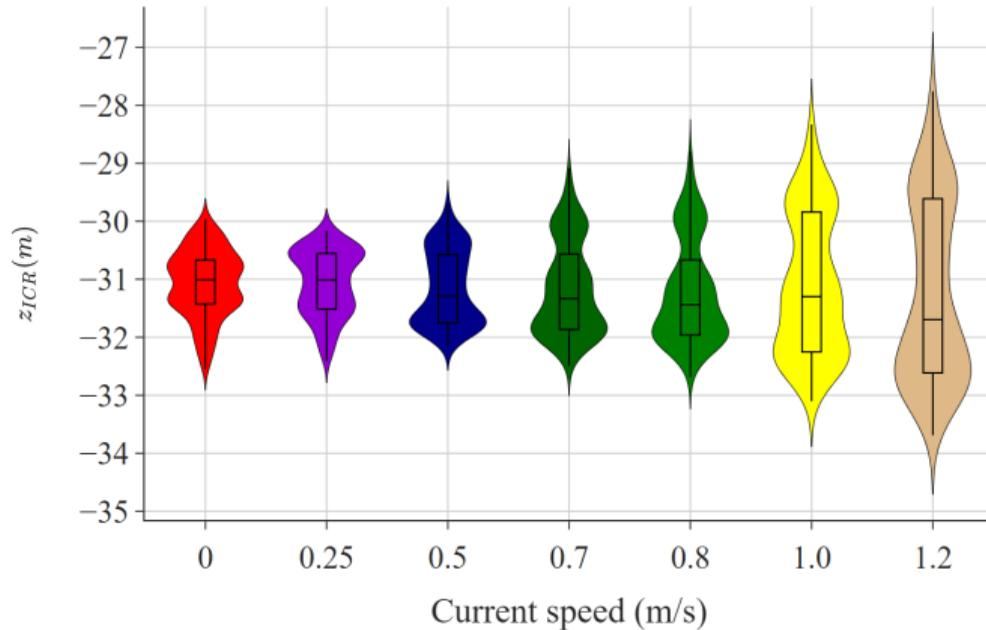
**Figure:** The ICR of FOWT in regular waves and current - distribution of z coordinate
