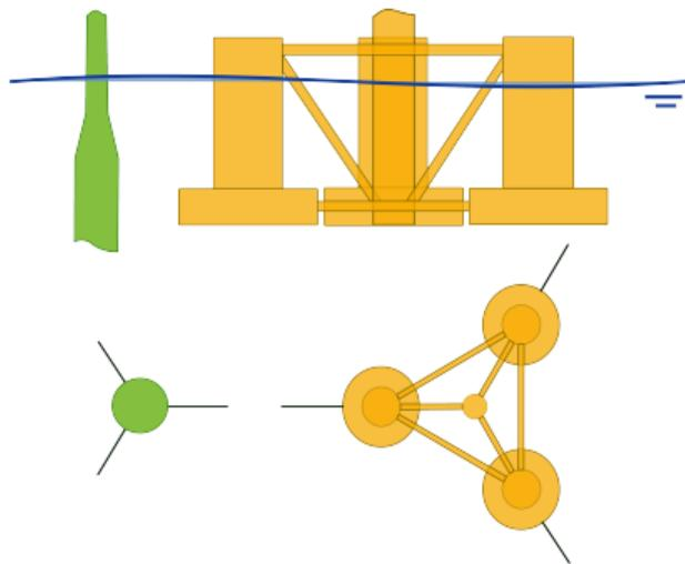
**Figure:** OC3 spar (left), OC4 semi (right)
