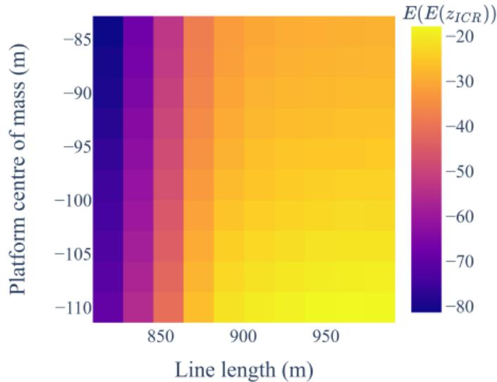
**Figure:** Design space - OC3 spar.
