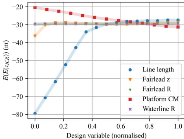
Figure: Sensitivity of  $z_{ICR}$  to spar variables
