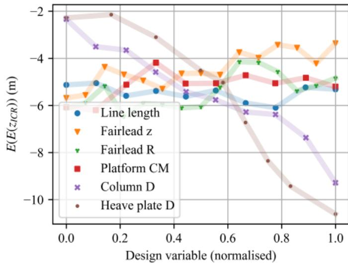
Figure: Sensitivity of  $z_{ICR}$  to semi variables
