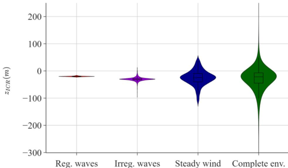
**Figure:** The ICR of FOWT in normal environment - distribution of z coordinate
