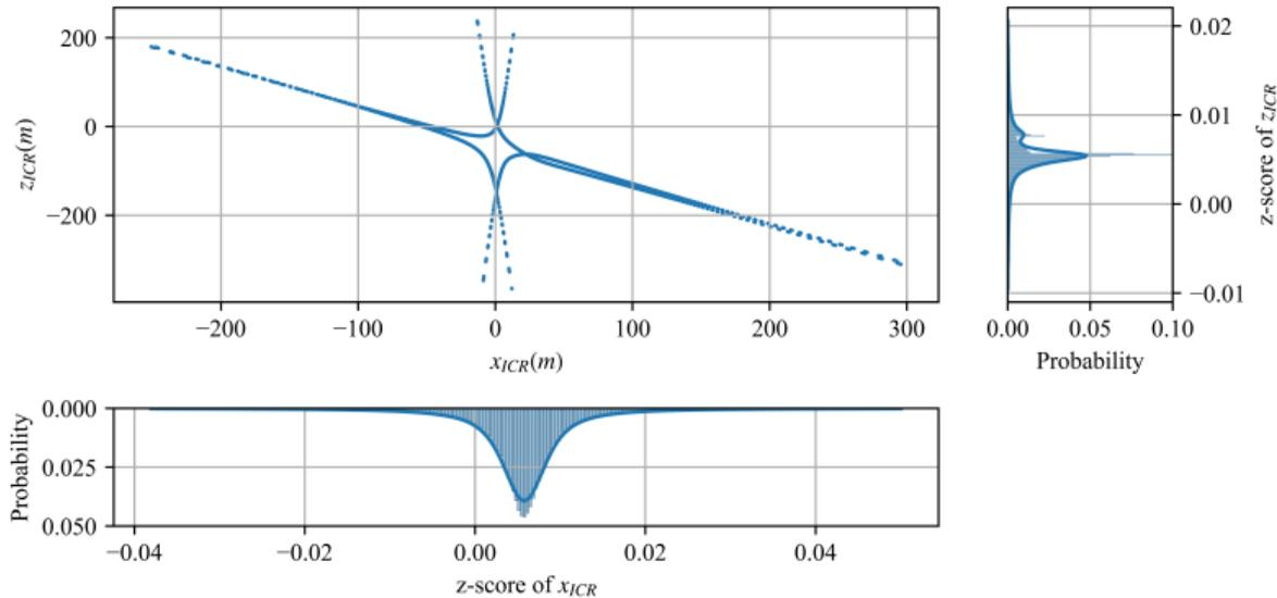
**Figure:** The ICR of FOWT simulated in regular waves - distribution of coordinates
