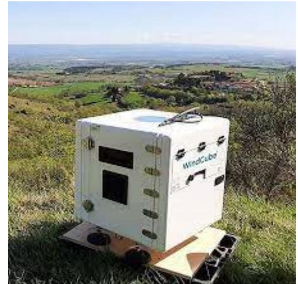
This study focuses on the pulsed fixed vertical lidar
