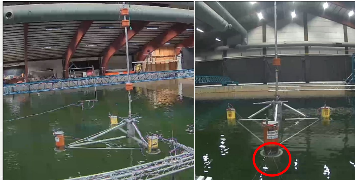
Video: Representation of floater motions after mooring line released for I8 wave case
