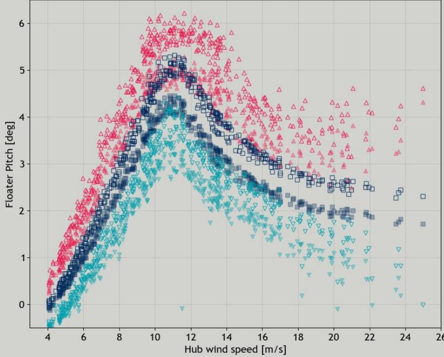
**Note:** Catenary system is more vertical which gives higher pitch restoring moment / smaller mean pitch angle
