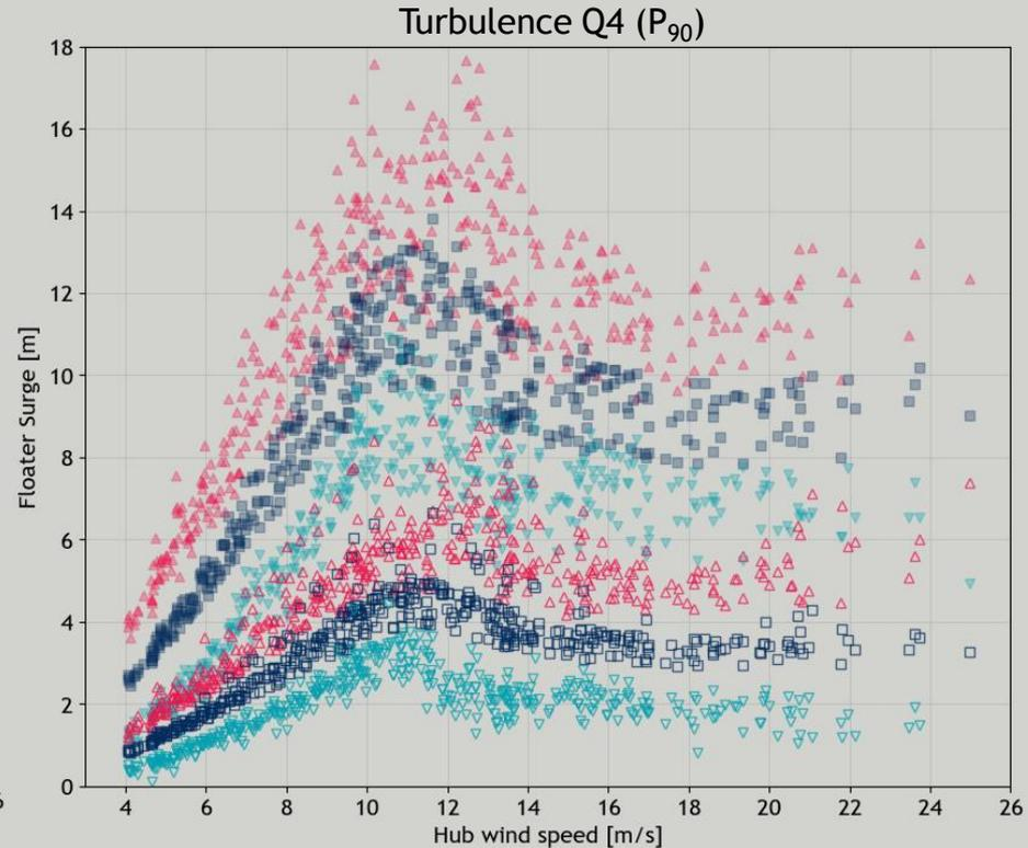
**Note:** Semi-taut run with half of rope permanent elongation which results in a stiffer system / less horizontal motion
