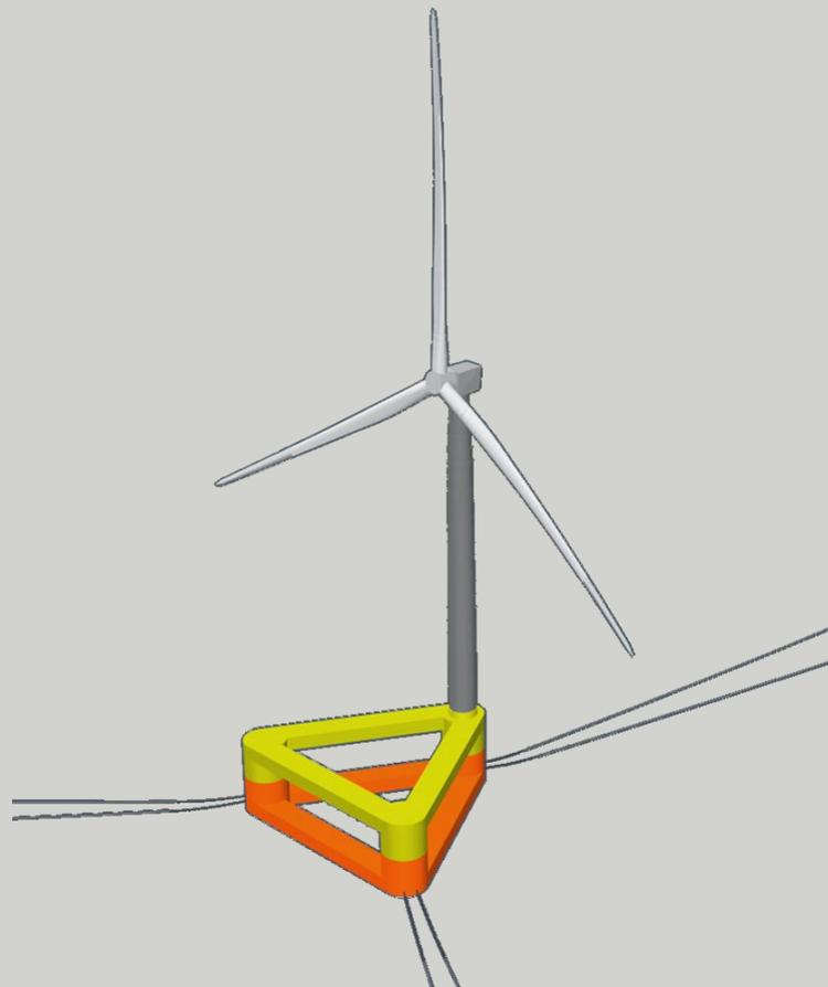
Fully-coupled analysis in OrcaFlex with Kaimal 3D turbulent wind from TurbSim
