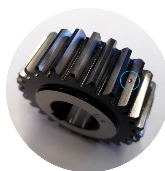
FIG.3: Left: Segment of the frequency spectrum (44th harmonic of the GMF at 24,232 Hz) Sonotec T20 sensor, n_{in} = 15,3 Hz, T_{out} = 24 Nm, pitting size 0,575 %, \eta = 81 mPas. Top: Pinion with manufactured pitting
