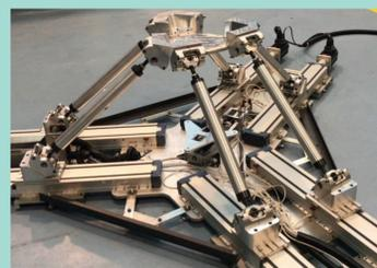
HexaFloat 6 d.o.f. floating motions tested on scaled HAWTs (LIFES50+ [2,3], OC6 Phase III [4]).
