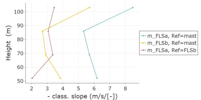
Figure 2: Regression slopes with inverted sign, describing the sensitivity to shear exponent of FLSa and FLSb using the mast and FLSb as a reference, for each measuring Lidar height.
