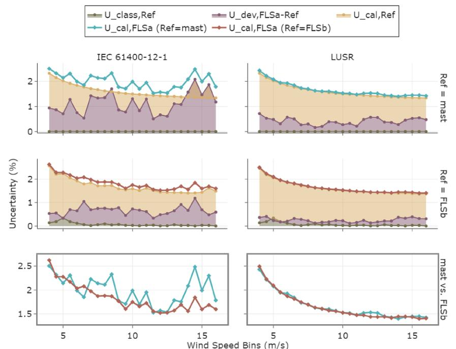
Figure 3: Calibration uncertainty sources of FLSa at the height of 103 m for each wind speed bin. Using IEC 61400-12-1 standard (left) and LUSR (right); using the met mast (top) and FLSb (middle) as a reference, and a comparison of both (bottom).
