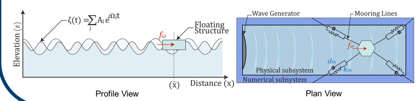
The first step in the experimental design is to estimate the low frequency added mass and damping parameters from a set of experiments  $i = \{1, ..., N\}$  with identical wave elevation profiles but different sets of mooring stiffness and damping values  $(k_m, d_m)$ :
