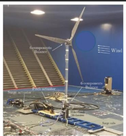
Figure 1: Polimi wind tunnel during the surge tests with scaled DTU-10MW RWT
