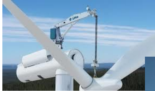
Liftra LT1200 - self-hoisting Crane
