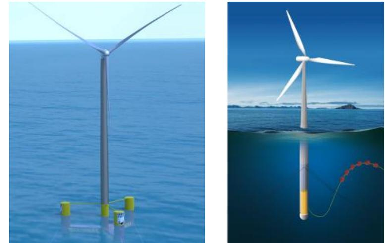
Figure 1 IEA 15MW reference wind turbine mounted on UMaine Voltturn US-S (left) and WindCrete (right) floating platforms
