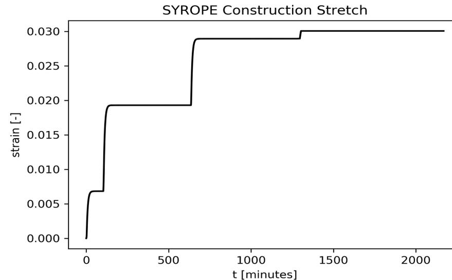
Each time the tension exceeds the previous max tension, the ratchet expands, and cannot compress again. This is a permanent elongation of the rope. The scale is arbitrary
