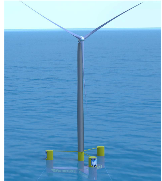
Figure 3. UMaine 15MW reference platform [3].
